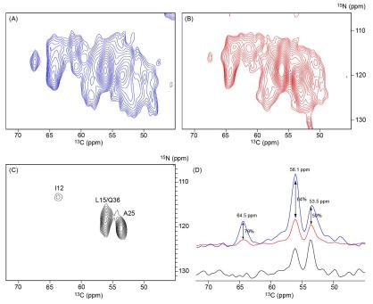
dimension at <sup>15</sup>N=120 ppm from 1(A) to 1(C) highlight differential reductions in resonance intensity from FDR dephasing, and the resulting difference spectrum.
