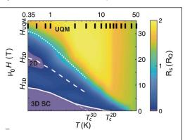
Fig.1 Interpolated color contour plot of the sheet resistance R<sub>s</sub> as a function of temperature and magnetic field. Black vertical marks indicate measurement temperatures. The regimes of 3D and 2D zero superconductivity with electrical resistance are labeled; the ultra-quantum metal phase occurs at fields above the dotted line. Characteristic fields  $H_{3D}$ ,  $H_{2D}$ , and  $H_{UQM}$
