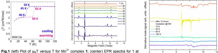
**Fig.1** (left) Plot of  $\chi_{M}T$  versus T for Mn<sup>3+</sup> complex **1**; (center) EPR spectra for 1 at temperatures in range 10-80 K at 336 GHz; (right) EPR spectra for Fe<sup>3+</sup> LIESST-active complex **2** at 240 GHz.
