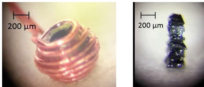
Fig.2 Pr_2Ir_2O_7 crystal in PDO coil (left) and stack of Nd_2Ir_2O_7 crystals (right).
