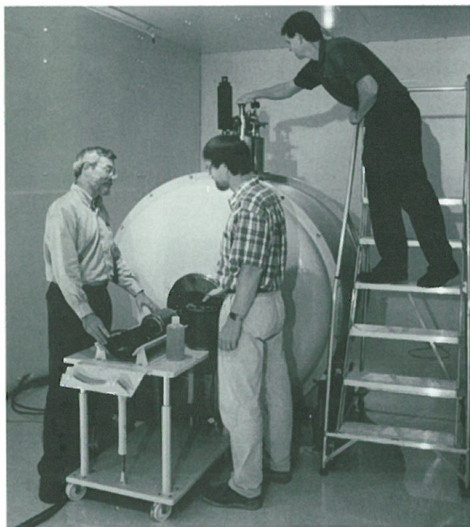
This 4.7 T, 330 mm bore magnet system is part of a small animal imaging spectrometer at UF.
