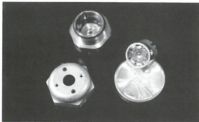
The largest of the diamond anvil cells, shown disassembled. The coin diameter is 19 mm.
