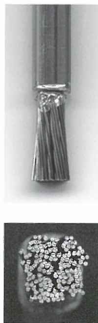
Figure 1. A typical CICC (cable-in-conduit- conductor).
