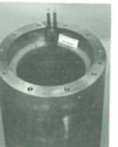
7. The fifth coil of the nested nine-coil quasi-continuous magnet. The complete magnet system will store 90 MJ when energized to 60 T.
