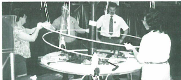
Figure 5. The NbTi coils, a pancake-style winding, are now at Everson Electric for insulation and VPI.
