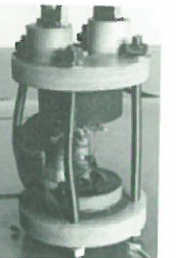
16. Prototype pulsed magnet tested to destruction to verify code predictions and test strengthening options.
