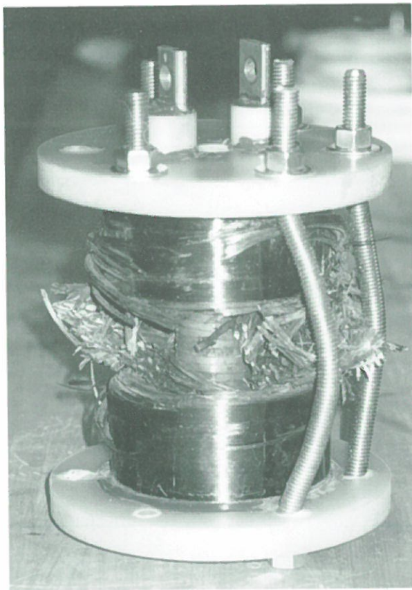
Figure 2. Pulse magnet after failure. It occurred due to mechanical overstressing of the conductor and the reinforcement caused by excessively high Lorentz forces.
