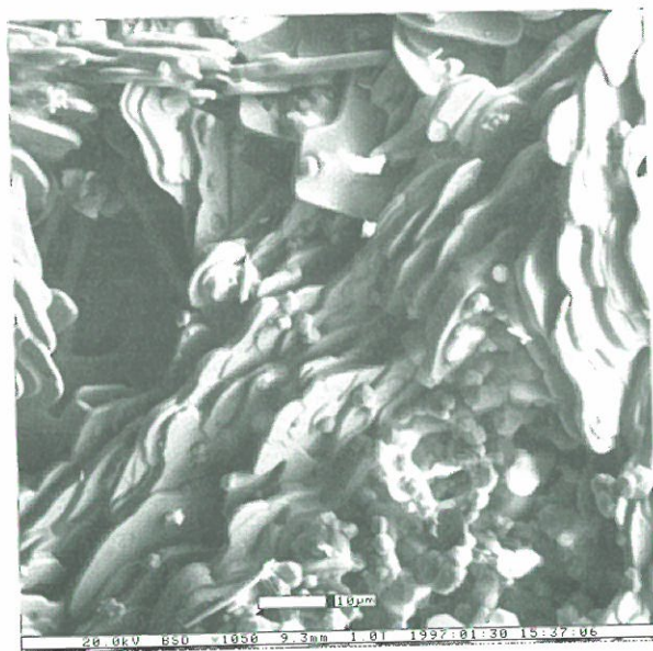
Figure 1. Scanning electron micrograph of Bi-doped Hg-1223 superconductor showing good grain growth and texturing.
