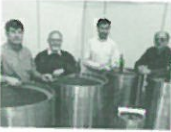
2. The complete set of nine coils for the 60 T quasi-continuous magnet are ready for nested assembly. From left to right are Jim Sims, Don Parkin, Larry Campbell, and Dwight Rickel.
