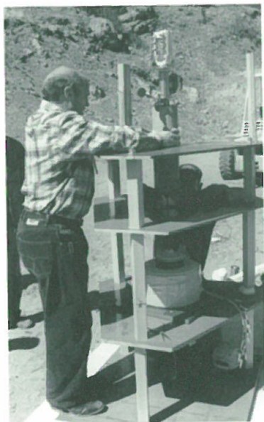
Figure 4. Bob Clark, Director of the National Pulsed Magnet Laboratory of Australia, carefully lowering the He-4 cryostat into the armed 1,000 T MC-1 flux compression generator during the Dirac series at Los Alamos.
