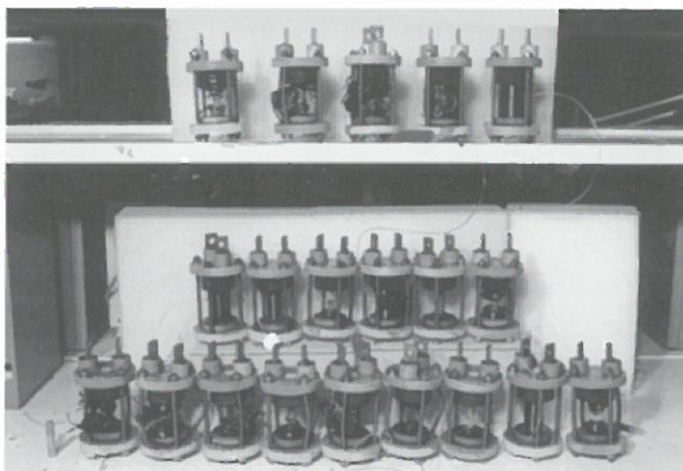
Figure 1. Two layer soft copper test magnets with varying reinforcement schemes after failure.
