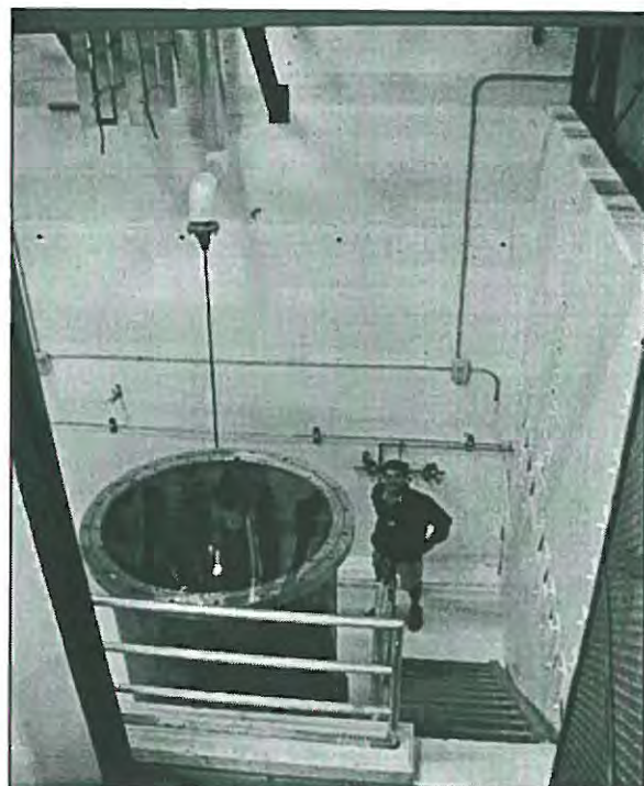
Figure 4. Postdoctorate Ross McDonald stands inside the magnet pit beside the new cryostat for the 100 T MS magnet.
