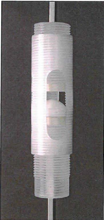
Figure 10. All dielectric photonic band gap resonator, tunable between 45 and 65 GHz. Development of this device is funded by the NHMFL In-House Research Program.
