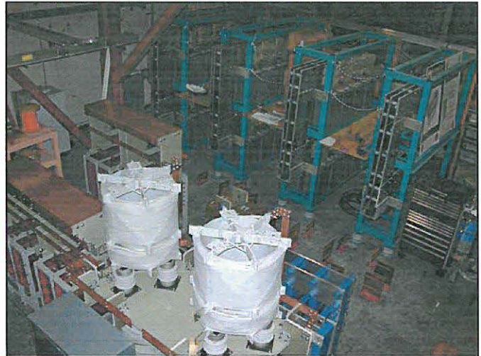
Figure 6. The 100 T magnet project's 2 mega-Joule capacitor bank is being built and will be operational in the spring of 2004.
