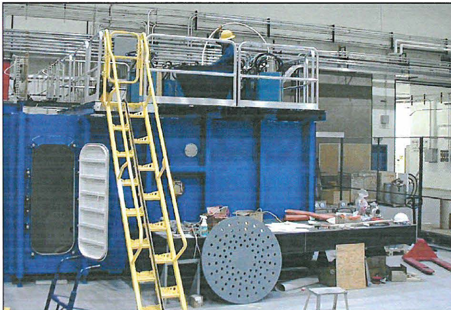
Figure 7. The single-turn magnet containment tank will house the 55 T pulsed magnet (milli-second duration) and the 300 T (micro-second duration) magnet system. The containment tank provides a safety barrier and control device for experiments on actinides and actinide compounds.
