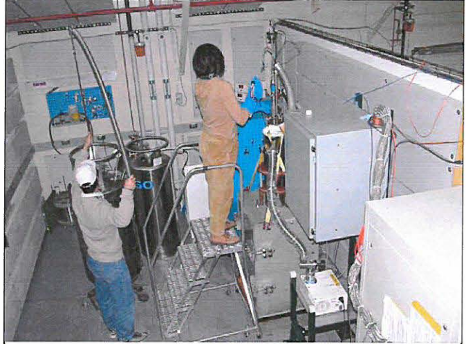
Figure 5. Users prepare for a liquid Helium transfer in cell 2 where the 50 T "mid-pulse" magnet is in operation. Due to the high volume of requests for use of this magnet system a second "mid-pulse" is now installed in cell 1.
