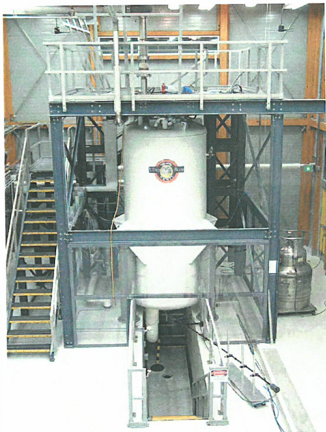
Figure 21. The NHMFL's 21.1 T, 105 mm bore NMR magnet is the product of a 13-year effort. It stands 16 feet tall, weighs over 30,000 pounds, and has a stored energy of 40 megajoules.
