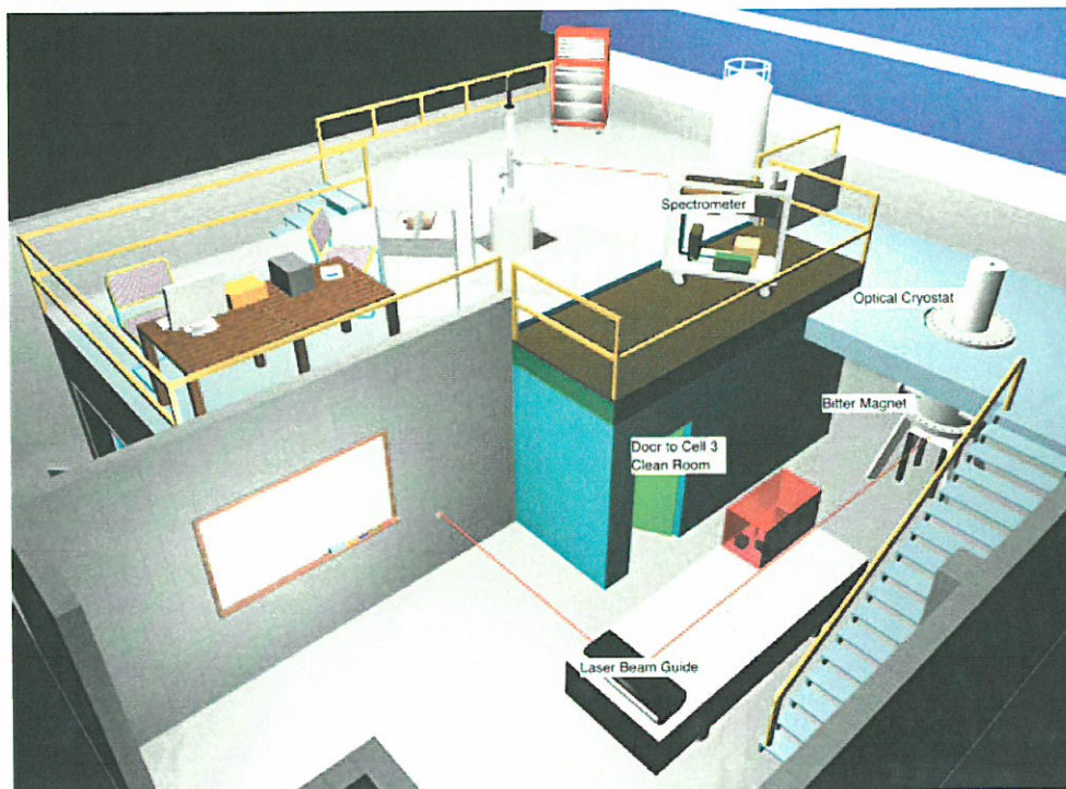
Figure 2. View of cells 3 and 5 with the new platform covering the clean room in cell 3.
