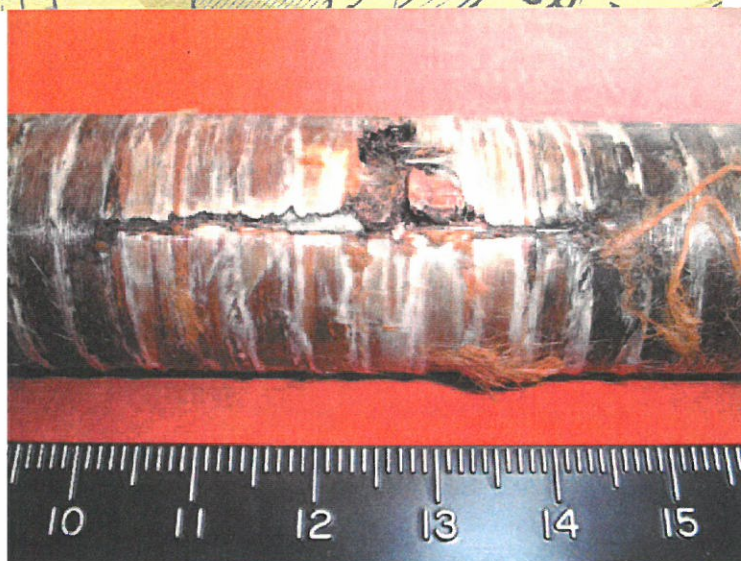
Figure 2. Layer 1 mid-plane fault illustrating short between turns.
