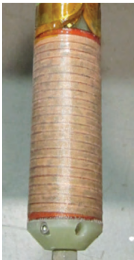
FIGURE 8. Layer wound coil with silk paper inter-layer insulation and glass fiber thread turn to turn insulation.
