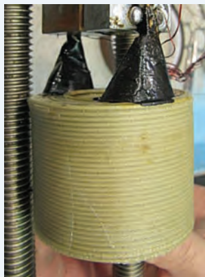
FIGURE 12. Small bore-tube-free coil tested successfully in the NHMFL 20 T Large Bore Resistive Magnet.
