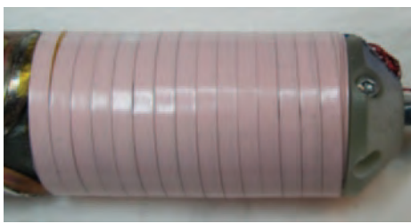
FIGURE 1. A coil wound with copper-plated conductor (4 mm wide) insulated with thin-walled heat-shrink tubing. This coil consistently generated 4.2 T in a 31.2 T background field, for a total of 35.4 T, a world record for superconducting coils.
