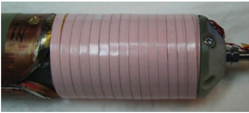
FIGURE 13. Layer-wound coil mounted on the probe. The coil is 64.5 mm long, with an inner diameter of 14.3 mm, and an outer diameter of 38 mm. The total length of conductor used is ~100 m.
