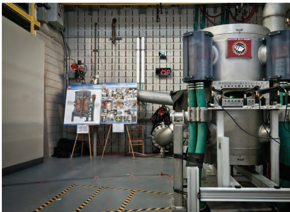
FIGURE 1. World Record 25 T Split Magnet at full field during the first user experiment in June 2011.
