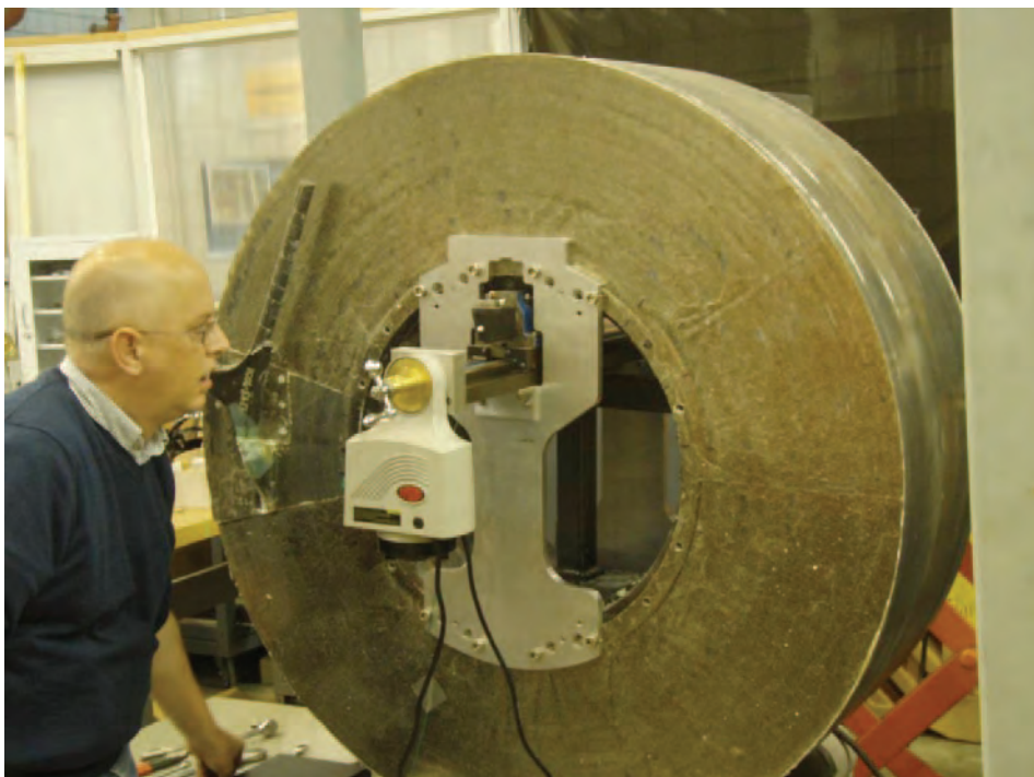
FIGURE 23. The CICC model coil after reaction heat treatment and epoxy impregnation. The flanges have been removed and a machining device is installed for removal of the coil mandrel.
