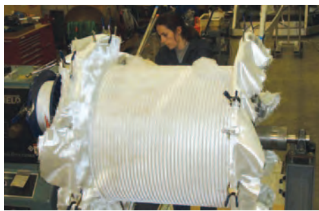
FIGURE 24. Winding of the HZB superconducting outsert coil.
