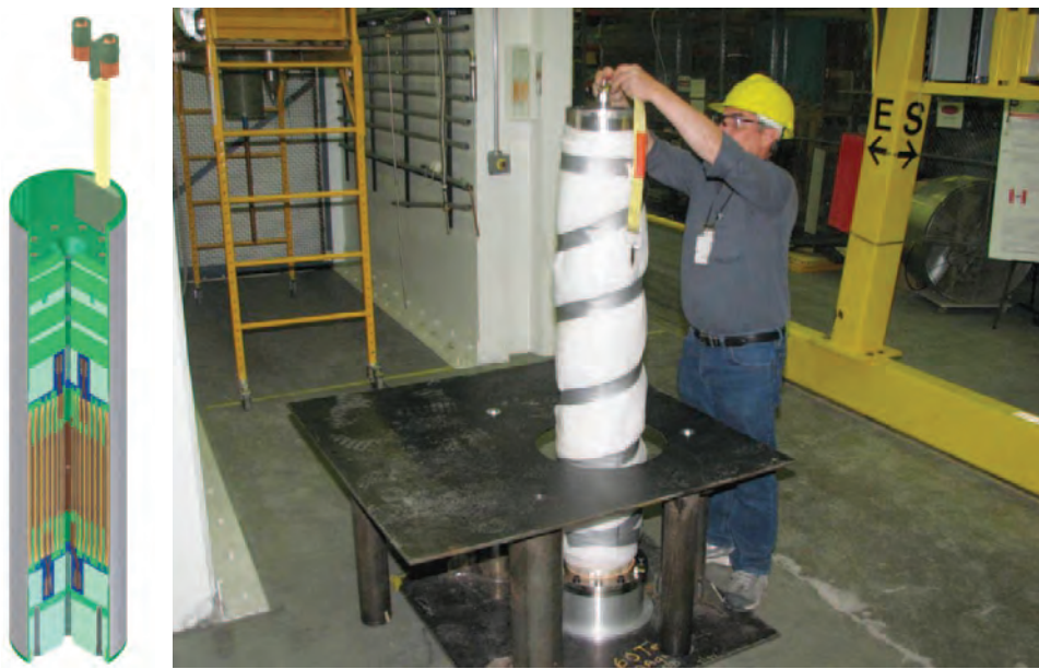
FIGURE 3. (Above left) Three-quarters section view of 10-mm insert upgrade magnet. FIGURE 4. (Above right) 10-mm insert upgrade magnet in final preparation.
