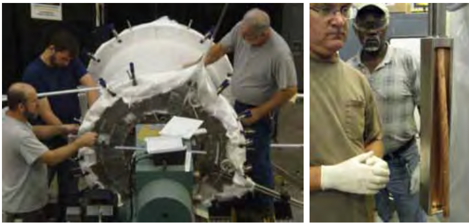
FIGURE 19. (Left) Winding of the FSU outsert CICC coil.
