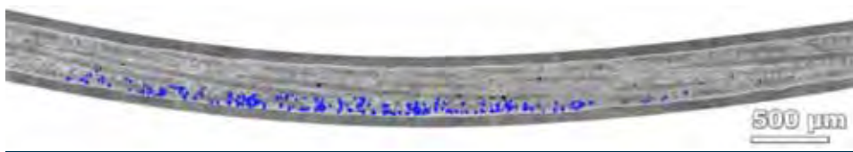
FIGURE 24. Longitudinal cross-section of a High Field Zone (HFZ) strand extracted from the Low-Pressure (LP) side of the CSIO1-2 SULTAN leg. The locations of cracks are shown in blue.
