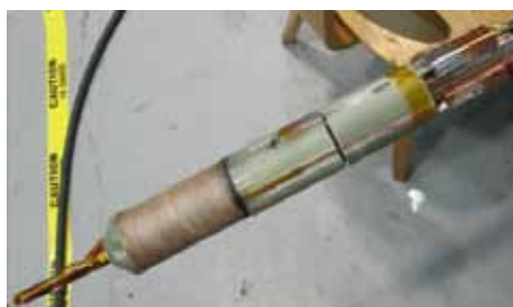
FIGURE 16. Bi-2212 layer wound coil mounted on the probe. The coil specifications are: 71.2 mm long, 14.3 mm ID, 36 mm OD, ~30 m total conductor length.
