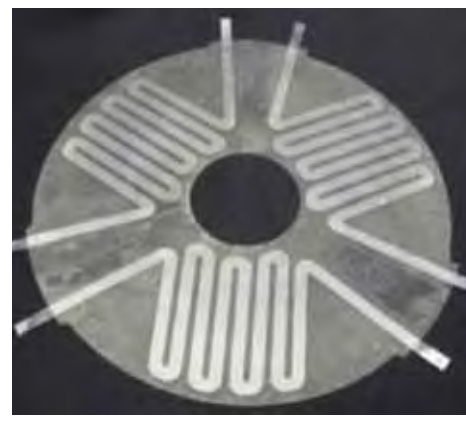
FIGURE 6. Quench protection heater consisting of stainless steel foils between thin epoxy-fiberglass sheets.
