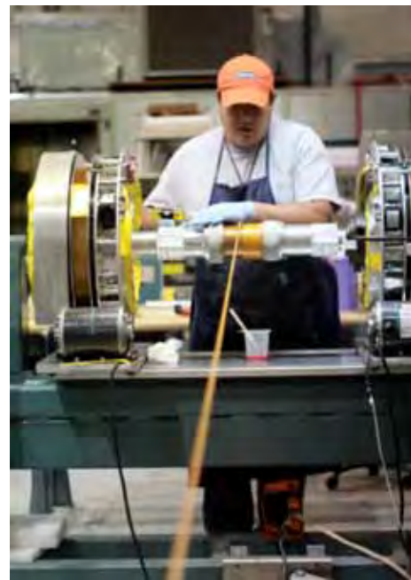
FIGURE 1. Technician James Michel of the NHMFL-PFF at LANL assembles a coil for the pulsed magnet user program.
