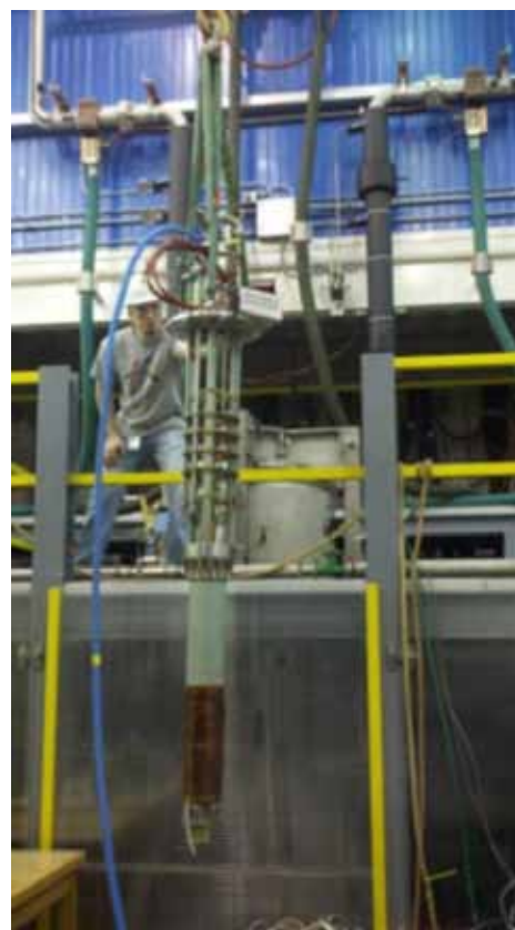
FIGURE 2. The prototype of the innermost coil of the 32 T all-superconducting magnet is raised prior to being installed in the dewar and tested.
