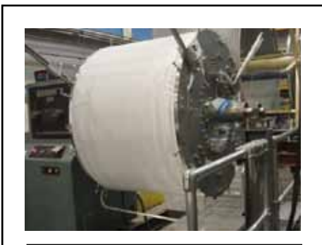
FIGURE 14. Wound CICC coil for NSF/FSU Series-Connected Hybrid magnet.
