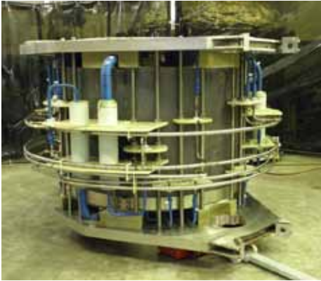
FIGURE 2. Nb 3 Sn Cable-In-Conduit Coil (cold-mass) for Helmholtz Zentrum Berlin ready for packaging and shipping. The FSU CICC coil will be identical.
