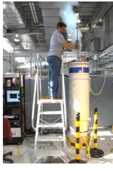
FIGURE 20. Testing of Nb 3 Sn wire for ITER at MagLab.
