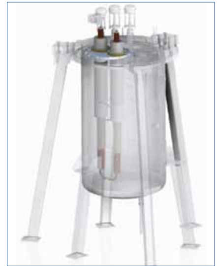
FIGURE 16. Nijmegen HFML Design of a Cryostat for Testing of the HTS Binary Leads.
