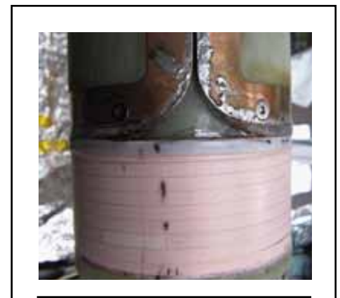
FIGURE 6. View of the layer wound REBCO coil and coil terminals [4].
