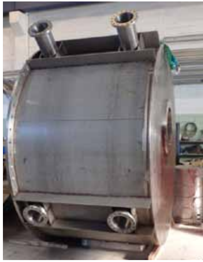
FIGURE 15. SCH Cryostat Vacuum Vessel with LN 2 Traced Bore Tube Thermal Shield in the Background.
