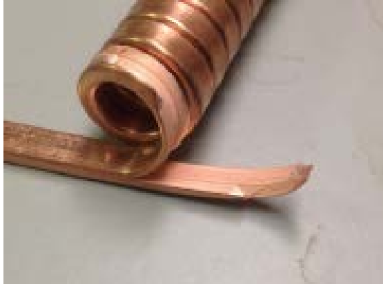
Figure 30: CuNb wire failed radius test.
