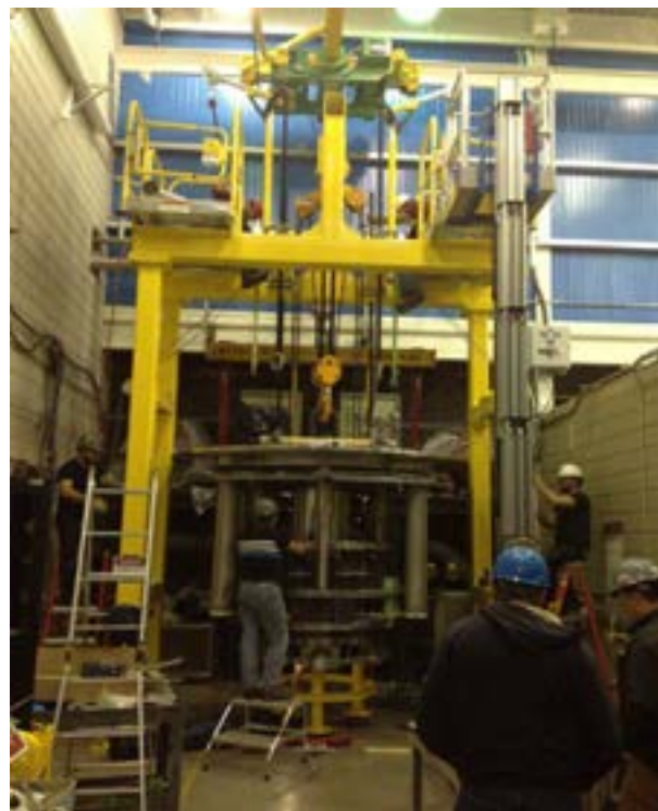
Figure 2: The 36 T hybrid magnet for FSU is entering the final assembly phase in cell 14 of the DC Field facility in Tallahassee. In early Feb. 2015 the 5.5-ton cold-mass was mated to the 6.5-ton cryostat for the first time.
