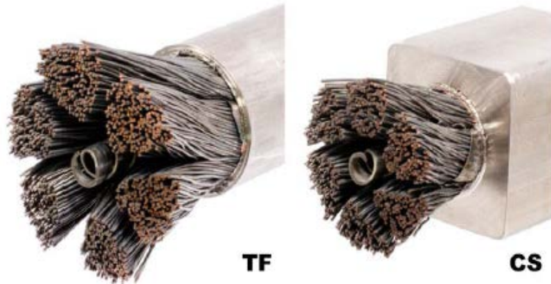
Figure 22: TF conductor (left) and CS conductor (right) with the jackets machined out and strands opened to show their transposition.
