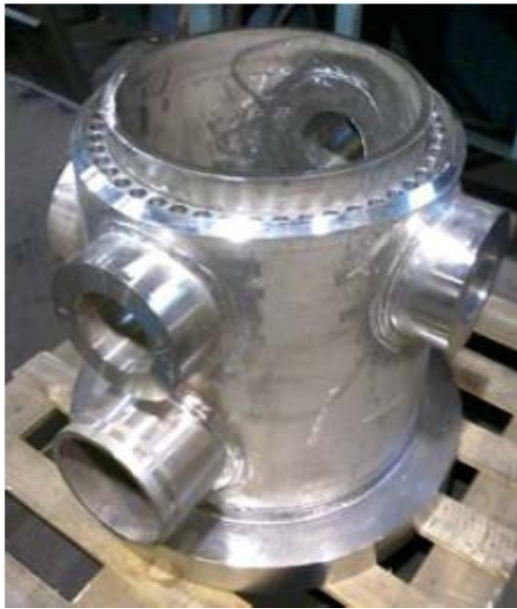
Figure 29: Snapshot of resistive housing during manufacturing (Hydrant 60% complete shown).
