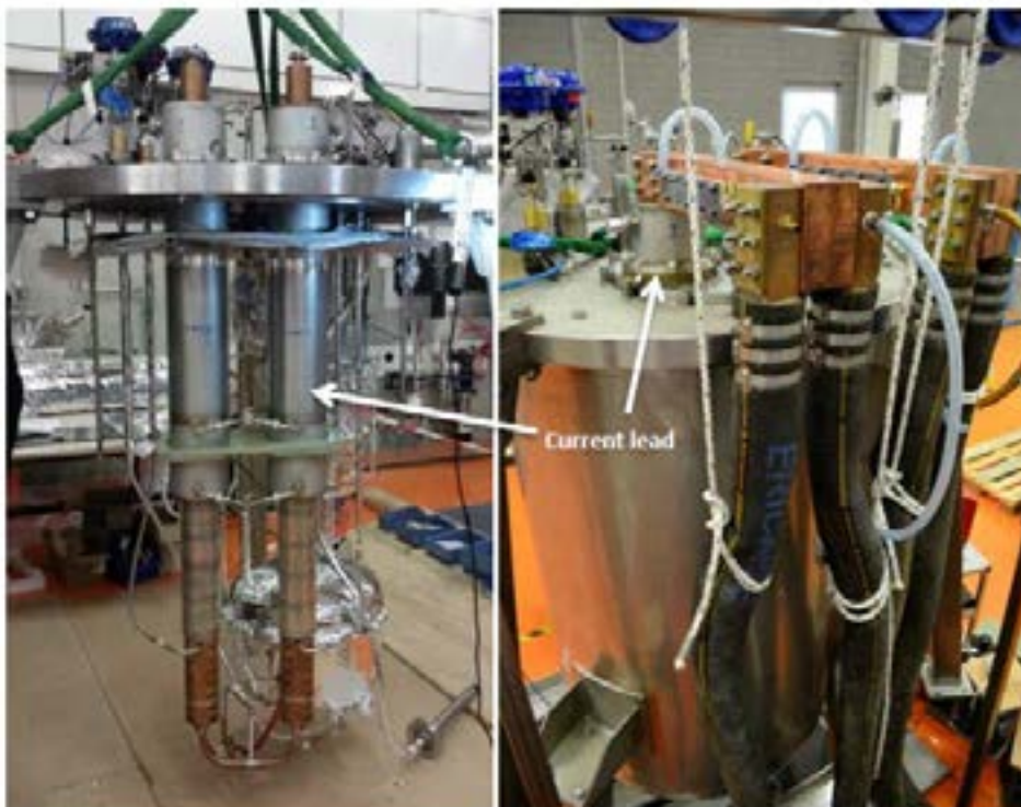
Figure 20: Testing of the cryostat and cryogenic system for the FSU/NSF SCH.
