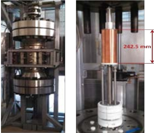
Figure 11: View of the new 100-bar overpressure furnace in closed (left) and open position (right) showing the full-size mock-up of the Platypus Bi-2212 coil mounted on a sample holder at the location inside the furnace where the actual coil will be heat-treated.
