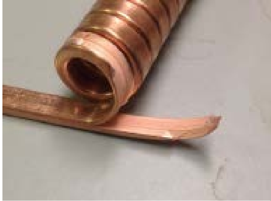
Figure 30: CuNb wire failed radius test.
