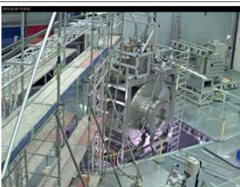
Figure 1: The 26 T hybrid magnet for HZB has reached full field and moved into the neutron guide-hall. Final system testing is expected in March 2015.
