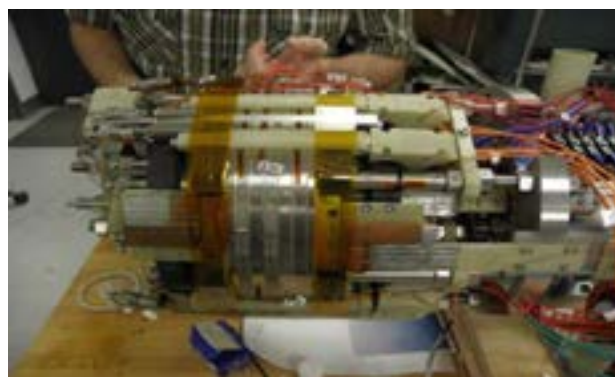
Figure 3: Prototype coils for the HTS section of the MagLab's 32 T all-superconducting magnet were quenched 80 times without degradation.
