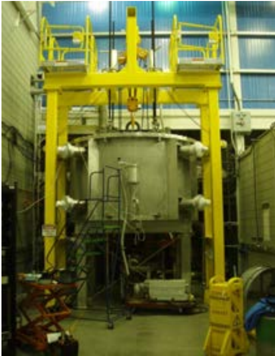
Figure 20: Testing of the cryostat and cryogenic system for the FSU/NSF SCH.
