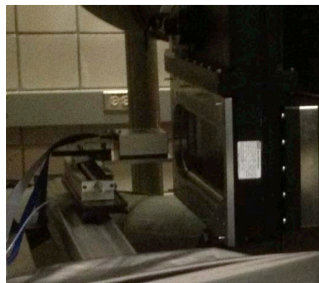
Figure 2: Dectris PILATUS3 detector mounted on a linear motion platform in front of one of the four scattering ports on the split helix magnet.
