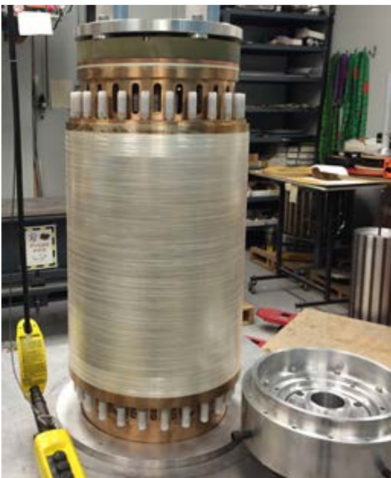
Figure 24: Snapshot of the completed resistive insert for the FSU-SCH (including 4 nested Florida-Bitter coils).
