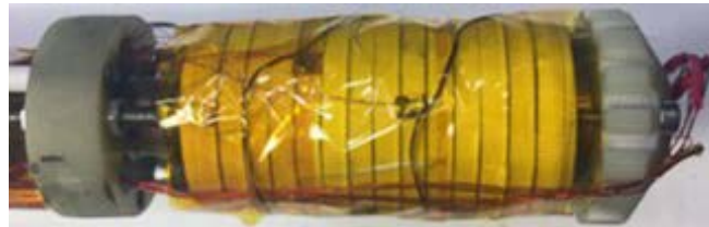
Figure 9: A picture of all-REBCO NI insert, which consists of a stack of 12 single pancake coils.
