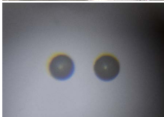
Figure 9 (a) A camera, a laser level (at the foreground) and a periscope (at the background) mounted at the hybrid platform. (b) The periscope and other parts of the optical setup mounted near the hybrid. (c) An image obtained by the setup described in text: two 1/16" balls located in the hybrid bore at ~11.5 T.
