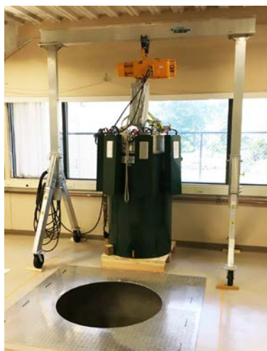
Figure 4.d.8: The 14T LTS background magnet made by Cryogenic LLC.
