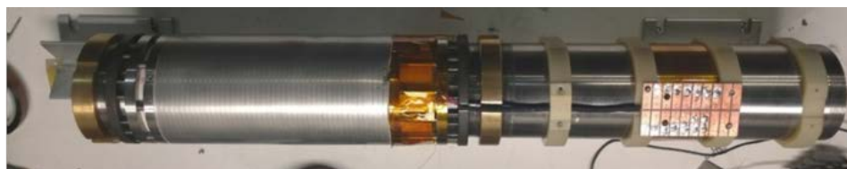
Figure 4.d.11: Bi-2223 test coil 'Tall-Thin' 1- The measured field homogeneity of the 'Tall-Thin' coil in the IMPDAHMA background magnet at 500 MHz was 116 ppm, which was in substantial agreement with the calculated homogeneity of 128 ppm.
