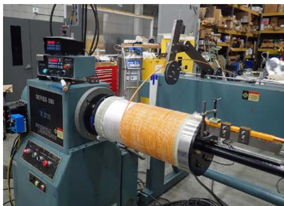
Figure 4.d.16: Winding of Coil #3 of the 100T Outsert.
