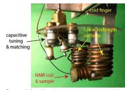
Figure 2.21: Ultra-low temperature double-resonance probe that was operated on Bay 2 for the study of one-dimensional <sup>3</sup>He.
