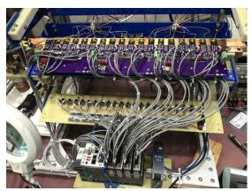
Figure 2.10: MOSFET bank testing setup.
