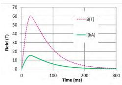
Figure 2.37: Proposed field vs time profile for the newly designed 60T mid-pulse magnet.
