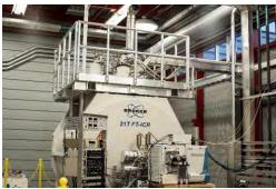
Figure 2.23: Picture of the 21T FT-ICR mass spectrometer.
