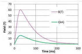
Figure 4.54: Waveforms of magnetic field and driving current for the 60T mid-pulsed magnet being developed at the PFF. At 60T the magnet pulse length of 60T pulses is about 300ms considerably longer than our standard capacitor driven magnets.
