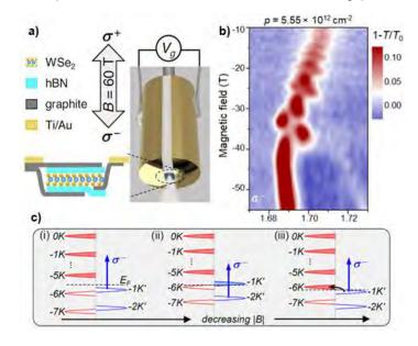
Figure 4.14: a) The WSe $_2$  monolayer-on-fiber assembly used for optical absorption studies in 60T. b) Discrete jumps in the absorption indicate emptying and spontaneous filling of specific valley LLs. c) Schematic depicting spontaneous valley polarization, driven by electron interactions.
