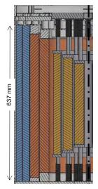
Figure 4.41: 40T Conceptual magnet design. REBCO sections in yellow; Nb<sub>3</sub>Sn in orange; NbTi in blue.
