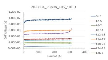
Figure 4.44: Voltage traces of consecutive layers in Pup-9 at 10T background field. The early transition somewhere within layers L8-11 is clearly visible.
