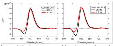
Figure 4.30: Subpicosecond intersystem crossing rate modulation at 25T.
