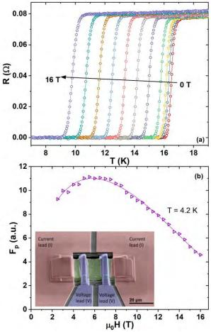
Figure 4.50: LTS-1. Superconducting characterizations of a Ta-Hf-doped Nb $_3$ Sn microbridge realized by "FIB"-ing the sample from the A15 layer of wire. The false-colored SEM image of the microbridge is shown in the inset. (a) Temperature dependence of resistive transitions at different magnetic field (data taken at 0 T, 0.5T, 1T, 2T and every 2T up to 16T). (b) Field-dependence of the pinning force Fp obtained at 4.2K
