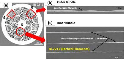
Figure 4.48: (a) Cross section of as-drawn wire showing three bundle types – tetragonal, pentagonal, and hexagonal. (b) and (c) Filaments extracted from as-drawn wire showing the varying filament area, which is particularly evident in the filament extracted from an outer bundle (b).
