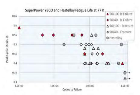
Figure 4.34 shows test results for fatigue of REBCO and Hastelloy tapes at 77K (load-control tension-tension fatigue, r= 0.1). In the legend, "X/Y" indicates REBCO composite tapes that include X microns of Hastelloy substrate and Y microns of copper cladding. "Ic failure" indicates the critical current dropped 10% or more. "Fracture" indicates the material broke.
