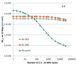
Figure 4.40: Inter-turn resistance versus cyclic loading of wet silver paint (Rc-303 and Rc-304) and stainless steel (No paint) when placed between two pieces of REBCO tape.
