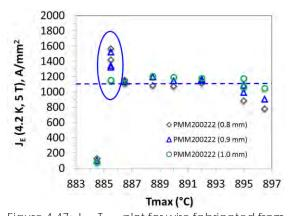
Figure 4.47:  $J_E - T_{max}$  plot for wire fabricated from Engi-Mat powder by B-OST. The plateau  $J_E$  is ~1100A/mm². The  $J_E$  peak is ~40% greater than the plateau.
