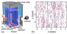
Figure 4.1: (a) A schematic diagram of our PTV counterflow setup. (b) Representative tracks obtained at 1.85K and 38mW/cm² for particles trapped on vortices (blue) and entrained by the normal fluid (red).
