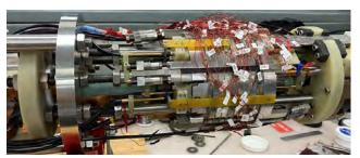
Figure 4.36: Assembled MTI-TC0 with instrumentation
