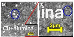
Figure 4.57: Scanning electron microscope image of the micro-structure of a present-day Cualumina conductor. The white spots in blue circles are (a) four micron-sized and (b) dozens of nanoscale alumina particles. For Cu+alumina to be suitable for use in a 120T magnet, this 500-fold variation in size must be reduced by eliminating the large particles.
