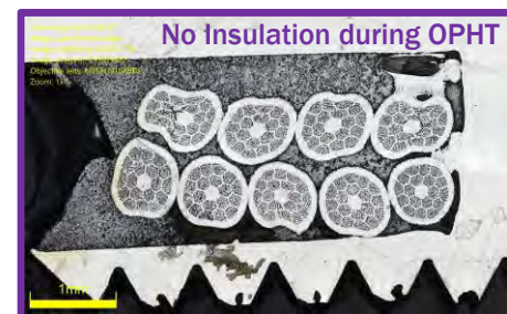
Figure 3. a) A typical cross section of one of the cables used in the coil. Several instances of leakage but also a certain amount of interfilamentary coupling are clearly visible. b) The cross section of the cable in the terminal area, where the alumino-silicate fiber was removed before the over-pressure heat treatment (OPHT), does not show any indications of conductor leakage.
