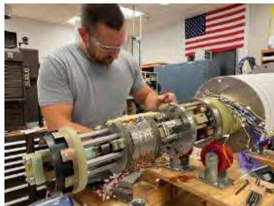
Figure 1. Installing the instrumentation wiring on TC2.
