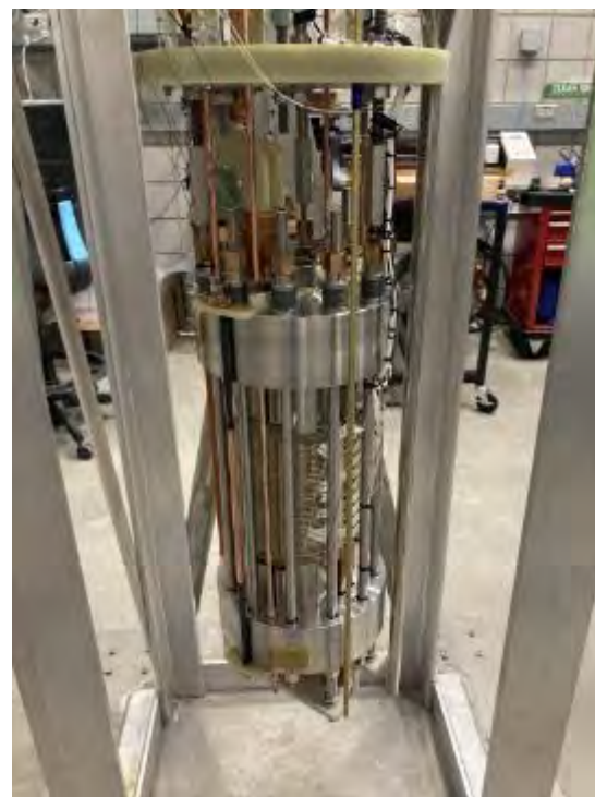
Figure 3. Test coil RI-NC after assembly.
