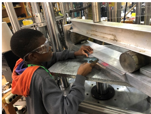
Figure 3.1.1: A Middle School Mentorship student in the MagLab's Materials Characterization Lab testing an I-beam.
