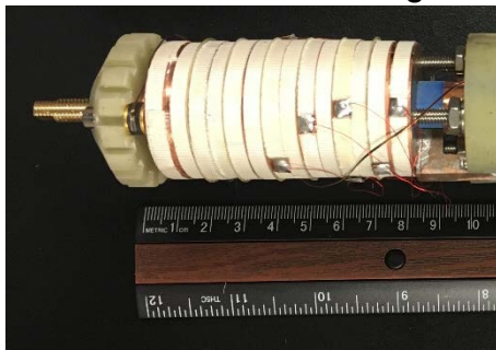
Figure 4.4.2: Photo of typical Little Big Coil. Two different ones were built and tested in 2019 to explore the quench dynamics in NI-REBCO coils.
