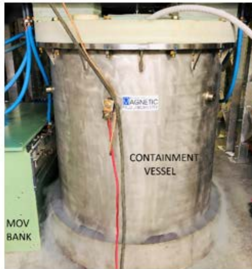
Figure 4.4.14: (Left) Measured waveform of magnet field generated by 75T duplex magnet during the commissioning phase, (Right) the picture of duplex magnet with MOV bank and containment vessel during its testing.
