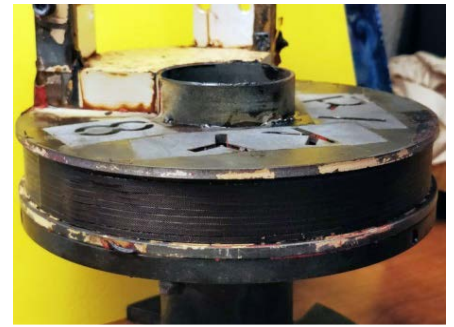
Figure 4.4.8: Test coil made with aspected conductor co-wound with high strengths alloy tape. This coil was strain limited when it exceeded the efficacy of the Inconel X-750 co-wind.
