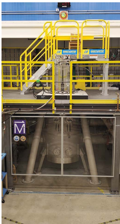
Figure 2.2.2.5: Cell 6 (41.5T) cryostat with advanced vibration isolation.
