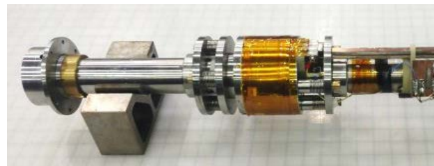
Figure 19: Test coil 'Short-Thick 1' and fixture
