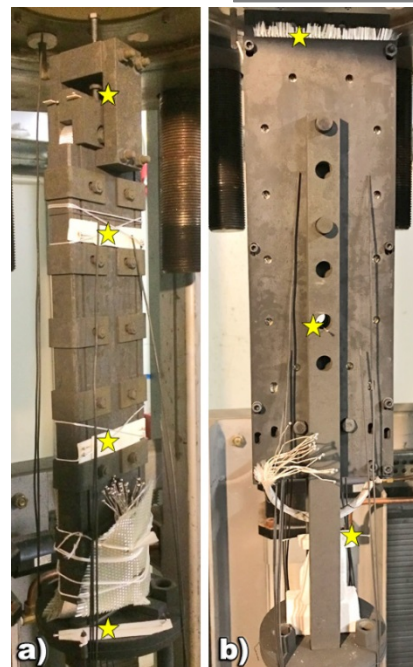
Figure 17: a) 'CERN/Twente' OPHT and b) 'LBNL RC3' OPHT. The yellow stars highlight positions of short witness samples.
