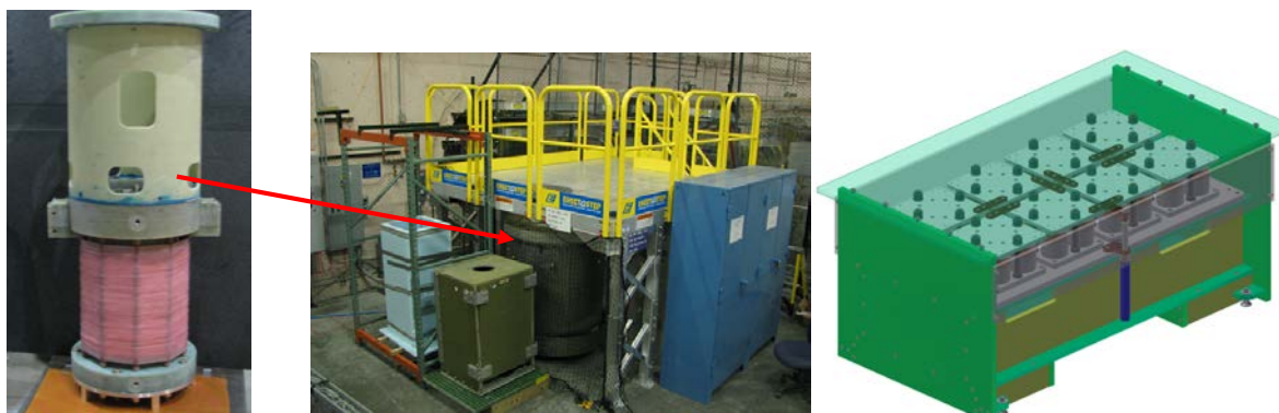
Figure 24: (left) Picture of the new duplex magnet built in 2017, (middle) the new duplex cell with user platform and the magnet cryostat housing, (right) illustration of the MOV bank.
