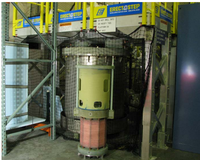
Figure 1: The new Duplex magnet sitting on the floor in front of the duplex magnet cryostat is housed in building 294 and will allow routine pulses up to 75 tesla for users in 2017.
