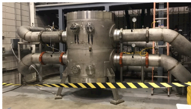
Figure 5: 41T resistive magnet located in cell 6.
