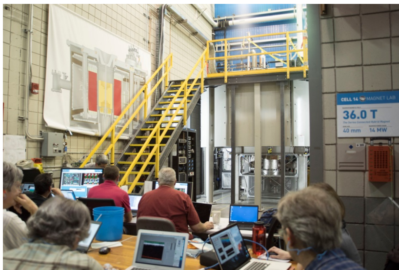
Figure 28: The Series-Connected Hybrid (background) with iron shield installed and personnel monitoring the system during magnet testing.
