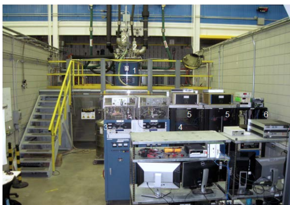
Figure 4: A Picture of Cell 4 with the 32 T magnet under test. 1: Cryostat; 2: Quench valves; 3 & 4: LTS and HTS magnet power supply respectively; 5: Battery banks to power quench protection heaters; 6: Rack with permanent electronics to monitor and safeguard the magnet. The hardware and screens in the front are for testing only and handle diagnostics.
