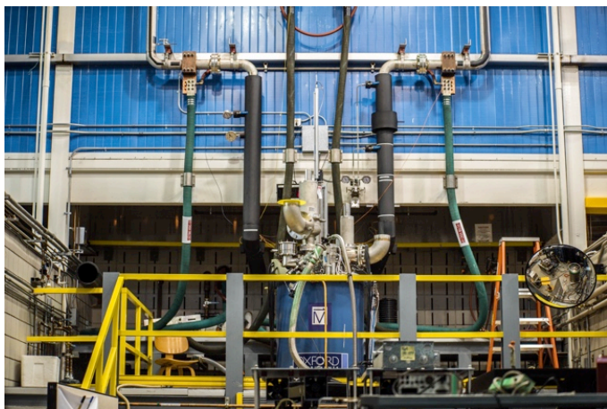
Figure 1: 32T superconducting magnet in its test stand.
