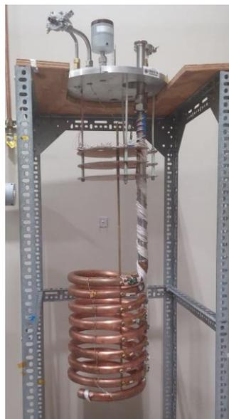
**Figure 2.** Internal assembly of helical tube system.
