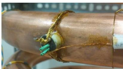
**Figure 3.** Stycast® epoxy encapsulated temperature sensor mounting on surface of helical tube system.
