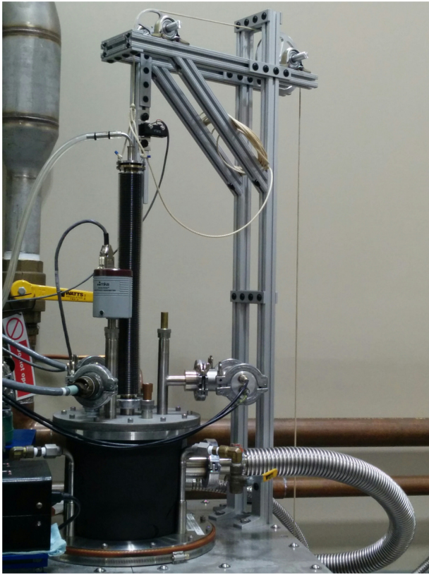
FIG. 4. Photograph of the top of the cryostat, showing the bellows and a portion of the pulling cable system.
