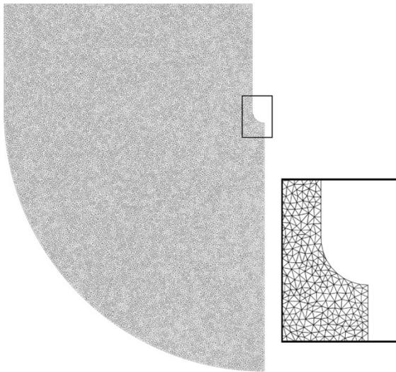
Fig. 4. Shape and fine FE mesh of the racetrack bore coil of Example 4. A quarter of the coil cross-section (on the left) and the bore fragment (at the bottom right) are shown. The mesh is excessively refined to maximize the computation accuracy.
