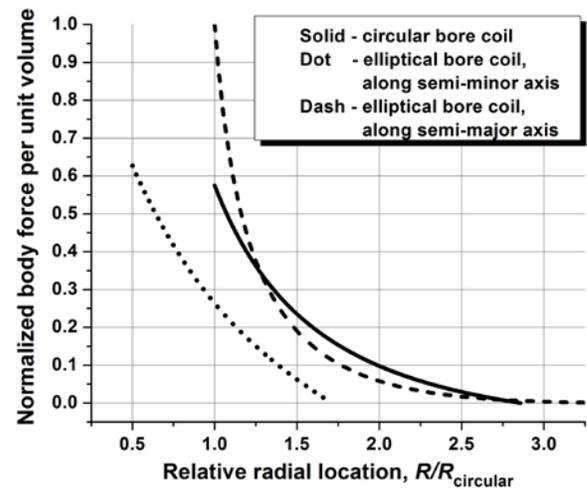
Fig. 5. Comparison of body force per unit volume in the elliptical bore and circular bore coils of Example 1.
