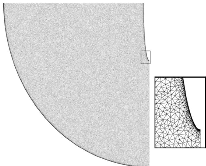
Fig. 3. Shape and fine FE mesh of elliptical bore coil of Example 3 (non-homothetic ellipses). A quarter of the coil cross-section (on the left) and the bore fragment (at the bottom right) are shown. The mesh is excessively refined to maximize the computation accuracy.
