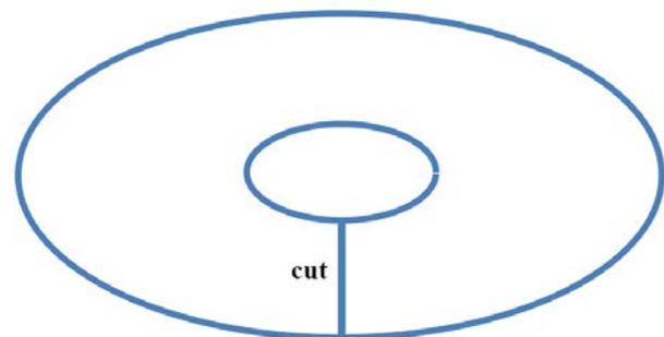
Fig. 1. Schematic of an elliptical Bitter disk / cross-section of an elliptical bore Bitter coil. The inner and outer ellipses are homothetic, with the short semi-axes significantly smaller than the long semi-axes. The cooling holes are not shown and not included in the analysis.
