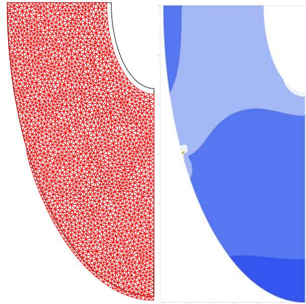
Fig. 7. The boundary of one fourth of an elliptical bore coil with no current versus the deformed mesh under current, with support (left), and the contour plot of von Mises stress (right). Rotated.
