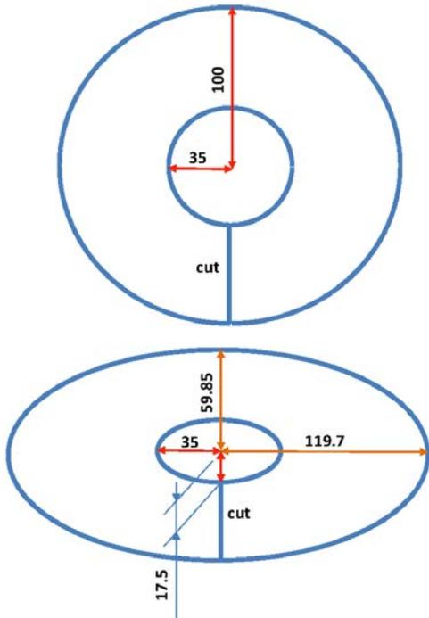
Fig. 2. Schematic and dimensions of Bitter disks of circular (upper) and elliptical bore (lower) Bitter coils of Example 1.
