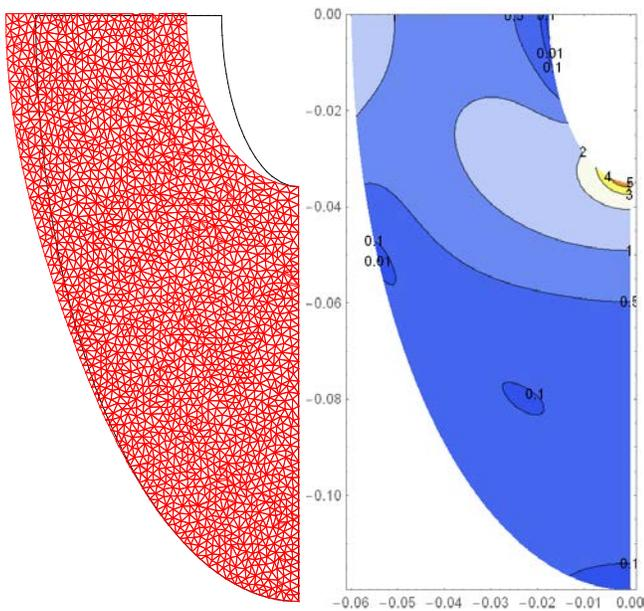
Fig. 6. The boundary of one fourth of an elliptical bore coil with no current versus the deformed mesh under current, with no support (left), and contour plot of von Mises stress (right). Rotated.
