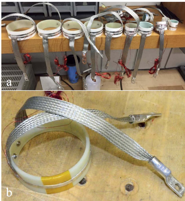
Figure 6. Single- and hard-way bent test-coil sections (a) and a curved splice sample (b).
