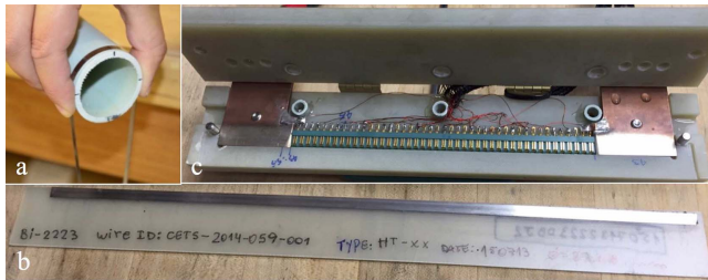
Figure 5. Single- and double-bend test procedure (a), straightened tape-sample after a single- or double-bend (b), and a clamp with a voltage-tap array to measure the I_c as a function of position at 77 K (c).
