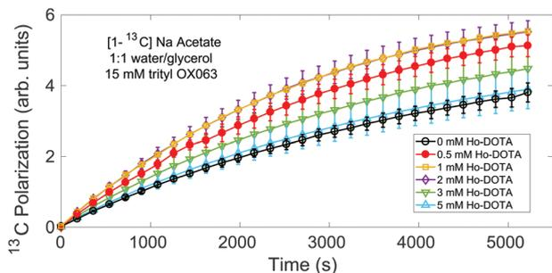
Fig. 2  $^{13}\text{C}$  polarization buildup curves of  $[1-^{13}\text{C}]$  sodium acetate in 1:1 (v/v) water/glycerol solution for different concentrations of Ho-DOTA (0, 0.5, 1, 2, 3, 5 mM) at the P(+) maximum peak position.
