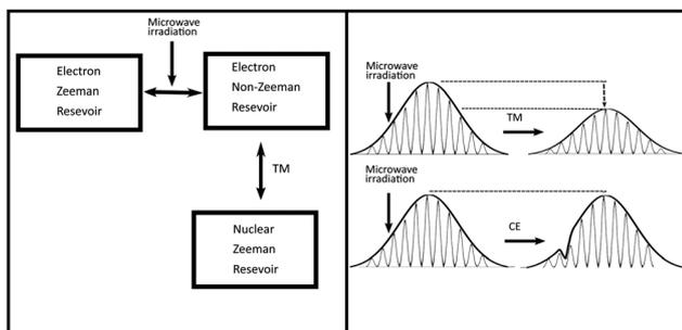
Fig. 3 Left panel: Schematic diagram of thermal mixing (TM), where a model of three interdependent spin baths is invoked. Right panel: The difference between the TM (complete saturation of the ESR line) and the cross effect (CE), where electron spectral diffusion is limited.
