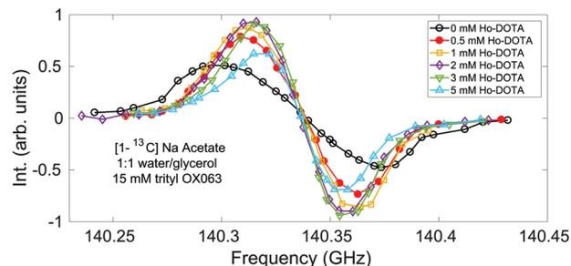
Fig. 1  $^{13}\text{C}$  DNP frequency sweeps of [ $^{13}\text{C}$ ] sodium acetate in 1:1 (v/v) water/glycerol solution in the presence of trityl OX063 radical for various concentrations of Ho-DOTA (0, 0.5, 1, 2, 3, 5 mM).
