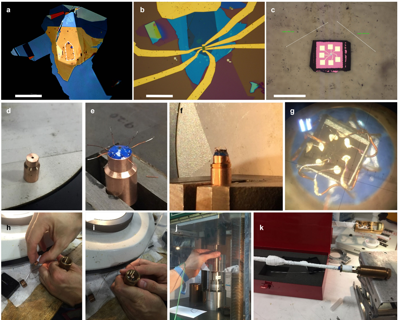
Extended Data Fig. 1 | Pictures of the set-up for pressure experiments. a , Graphene (outlined in white dashed line) is encapsulated between BN and placed on a graphite back gate. b , The device is shaped into a Hall bar and contacted for electrical measurements. c , The Si wafer is diced to approximate dimensions of 2\text{ mm} \times 2\text{ mm} . d , A new pressure cell stage. e , The stage is threaded with wires which are epoxied in place. f , The sample is glued to the top of the stage. g , Wires are connected to the device
