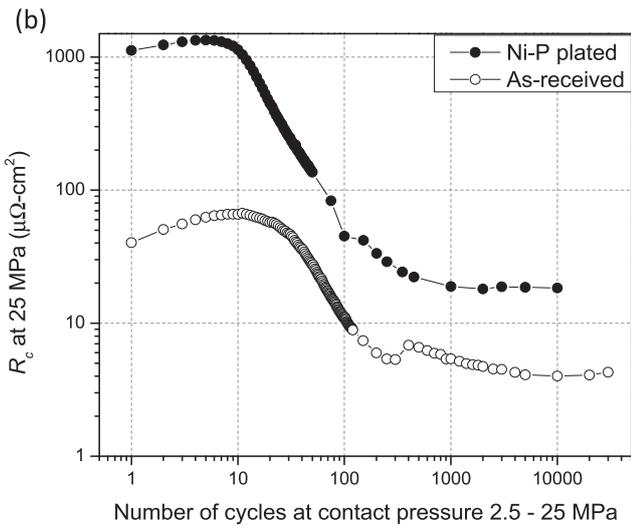
**Figure 6.** Effect of Ni–P plating. Ni–P is plated on REBCO with a 1  $\mu\text{m}$  pure Ni buffer layer (a)  $R_c$  versus Ni–P thickness. (b)  $R_c$  versus load cycles for 1  $\mu\text{m}$  Ni–P plated sample with an as-received sample for comparison.
