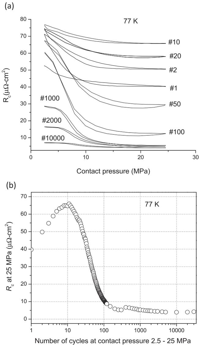
**Figure 2.**  $R_c$  of as-received SuperPower SCS4050 at 77 K. (a)  $R_c$  versus contact pressure curves for different numbers of load cycles. (b)  $R_c$  measured at 25 MPa as a function of number of load cycles.
