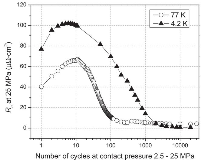
**Figure 3.**  $R_c$  measured at 25 MPa as a function of number of load cycles at 77 K and 4.2 K.
