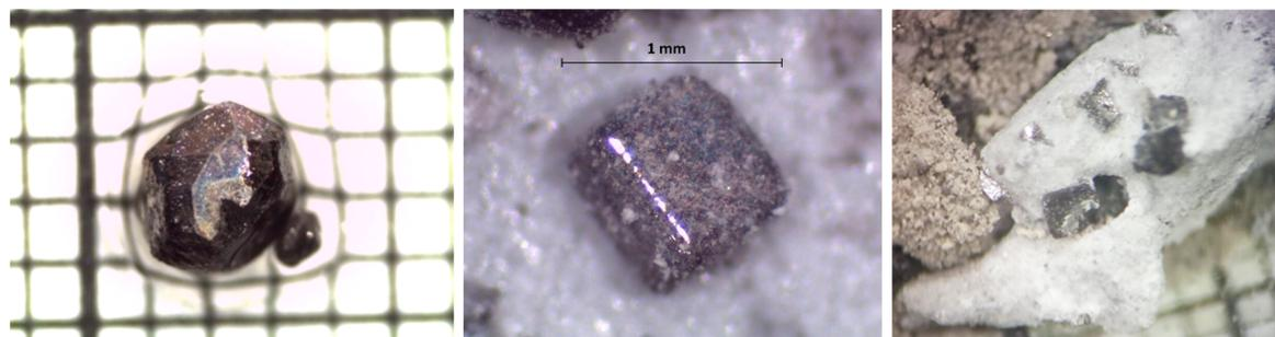
**Figure 1.** Microscope images of  $U_8Al_{19}Si_6$  crystals grown from aluminum flux. (a) The single crystal used for neutron diffraction experiment under Parabar oil on 1 mm grid paper. (b) A cuboid crystal showing aluminum oxide residue after NaOH etching. (c) Crystals growing off of a piece of alumina cement.
