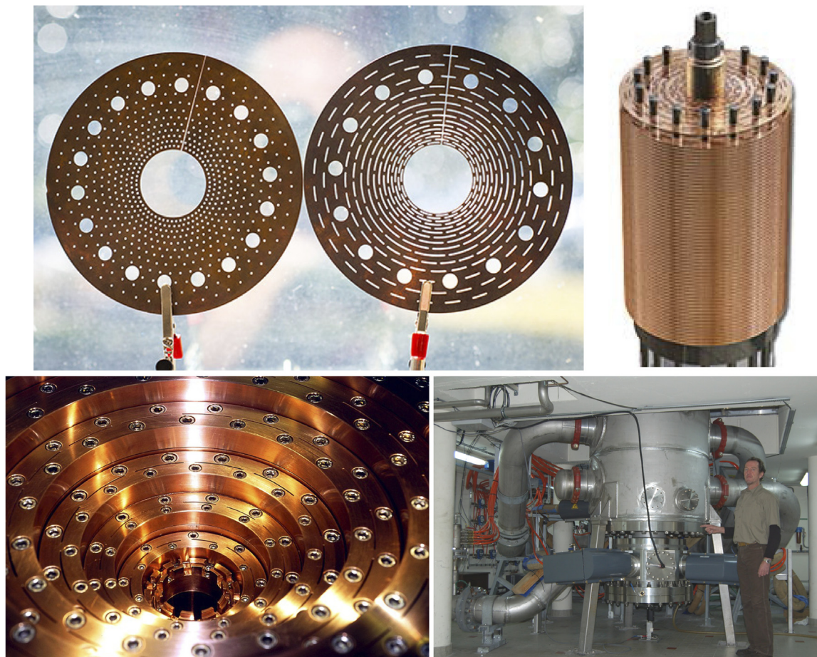
Fig. 19. Top left: Images of the original “Bitter-plate” design (round holes) and the more recent “Florida-Bitter-plate” design (staggered oval holes), used in the construction of high-field resistive electromagnets. The holes in the plates allow for the efficient flow of cooling water through the magnet, which is needed to dissipate the considerable (10s of MW) resistive heating. The central hole in the plates is about 40 mm in diameter. Top right: these plates, with separating insulating layers, can be stacked in a helical configuration to construct a complete magnet. Photos courtesy NHMFL. Bottom left: top view of a polyhelix assembly used in Grenoble to produce 37 T in a 34 mm bore. Bottom right: the 37 T in 34 mm/24 MW magnet at LNCMI-Grenoble using the polyhelix technology for the inner coils.
