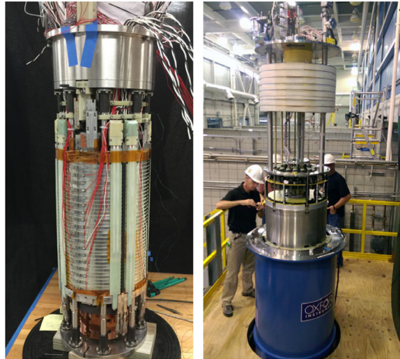
Fig. 23. Left: photograph of the innermost two high-Tc-superconductor (YBCO) coils of the all-superconducting 32 T magnet, whose successful operation was demonstrated in December 2017 at the NHMFL-Tallahassee. Total height of the pictured assembly is about 1 m. These YBCO coils are integrated within an outer coil set made of conventional (low-Tc) superconducting wire. The LTS outsert and the cryostat were designed and developed by Oxford Instruments NanoScience. Right: magnet assembly.
