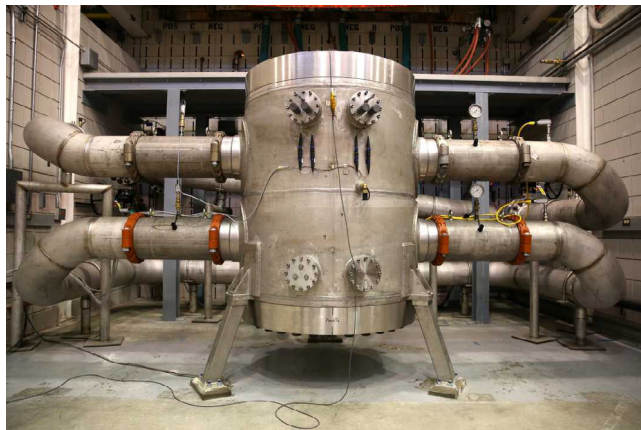
Fig. 20. Photograph of the 41.4 T resistive magnet at the NHMFL-Tallahassee (August 2017). This magnet is about 2 m in height, has a 32 mm bore and is powered with a 32 MW power supply. Its design is based on Florida-Bitter plates (see text) using high-strength copper–silver-alloy conductor. Source: Photo courtesy of the NHMFL-Tallahassee.
