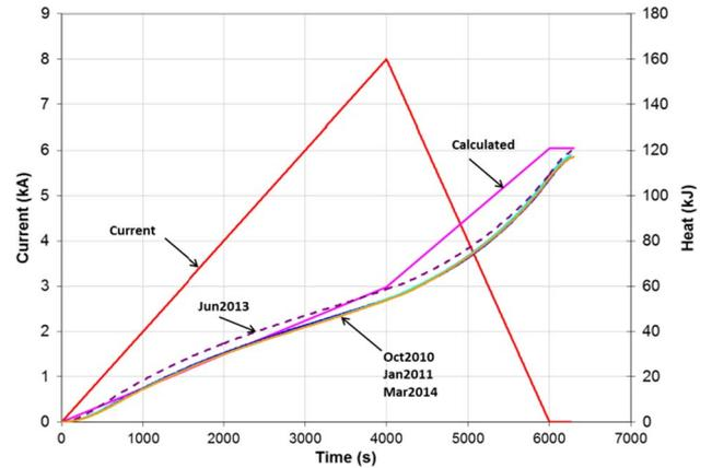
Fig. 4. Corrected heat deposition of the first ramps in October 2010, January 2011, June 2013, and March 2014. The four curves are almost laid over each other, and no substantial changes were observed for the four tests.
