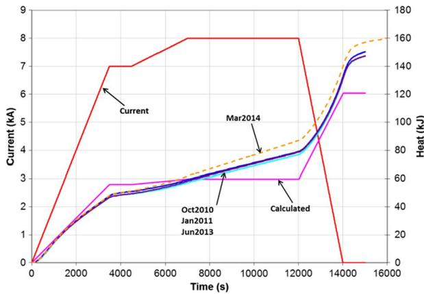
Fig. 6. Corrected heat deposition of the second ramps in October 2010, January 2011, June 2013, and March 2014. The test in March 2014 showed a bigger heat loss, and this may be caused by the new base temperature since it was lower than that in the past after the new cryogenic system was connected to the 45-T hybrid.
