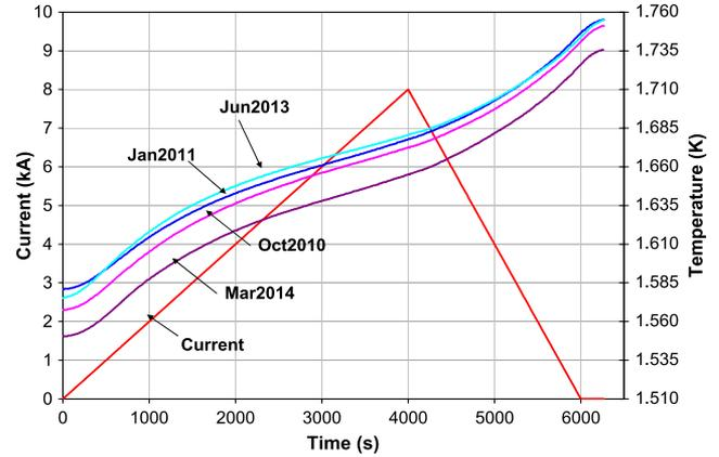
Fig. 3. Temperature response of the first ramp of the index heating tested in March 2014, compared with that in October 2010, January 2011, and June 2013. The current operation temperature of outsert (2014) is lower than that in the past after the LR280 was connected to the hybrid.
