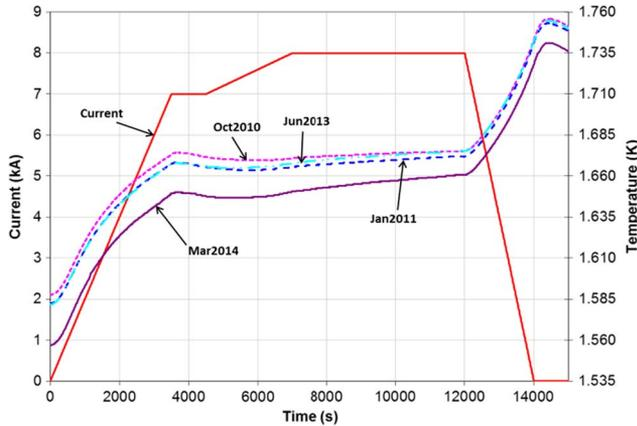
Fig. 5. Temperature response of the second ramps in October 2010, January 2011, June 2013, and March 2014. The temperature curves between 2010 and 2013 are almost the same. The temperature in the test of 2014 was lower than that in the past.
