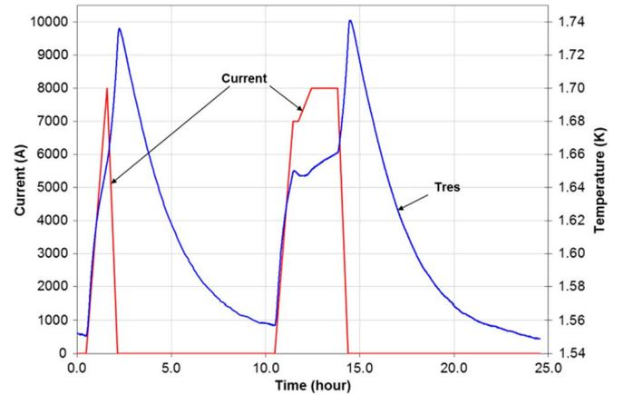
Fig. 2. Current of the outsert and the temperature response in the He-II reservoir ( $T_{\text{res}}$ ) during ramping of the 45-T hybrid outsert. The maximum operating current is 8 kA to achieve 11.5 T.
