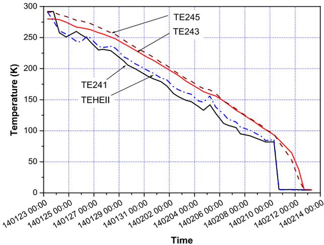
Fig. 1. First cooldown after upgrade of the cryogenic system for the 45-T hybrid. TE241 is the supply helium temperature, and TE245 is the return helium temperature during cooldown. TEHeII is the temperature in He-II bath. TE243 is the temperature of the magnet vessel. After cooldown, all the four sensors are immersed in liquid helium. The format of time shown in the  $x$ -axis is in a sequence of Year (2014), Month (01 is January and 02 is February), Day, Hour, and Minute.
