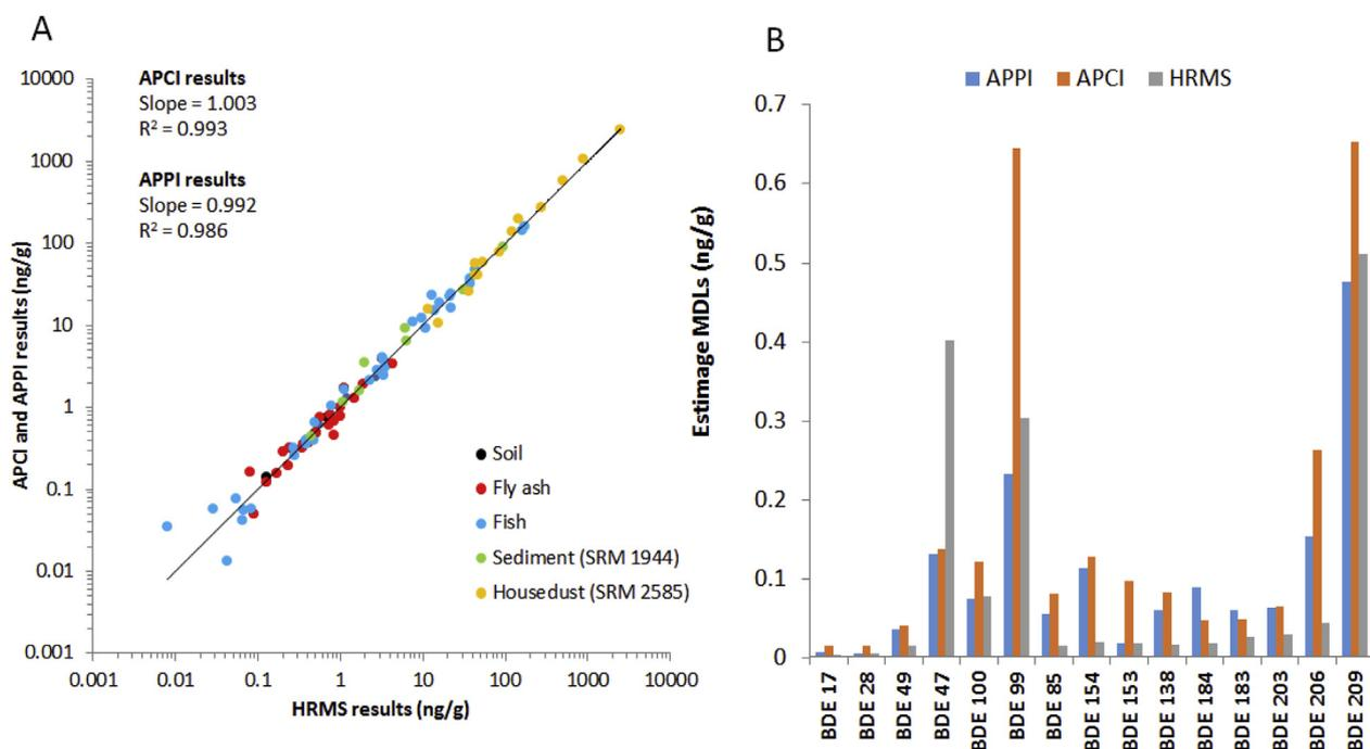
**Fig. 6.** (a) Comparison of PBDE concentrations in environmental samples obtained using GC-APCI and GC-HRMS; (b) Comparison of method detection limits for soil/sediment analysis of PBDEs obtained using GC-APPI, GC-APCI and GC-HRMS (MECP Method E3430 [35]).
