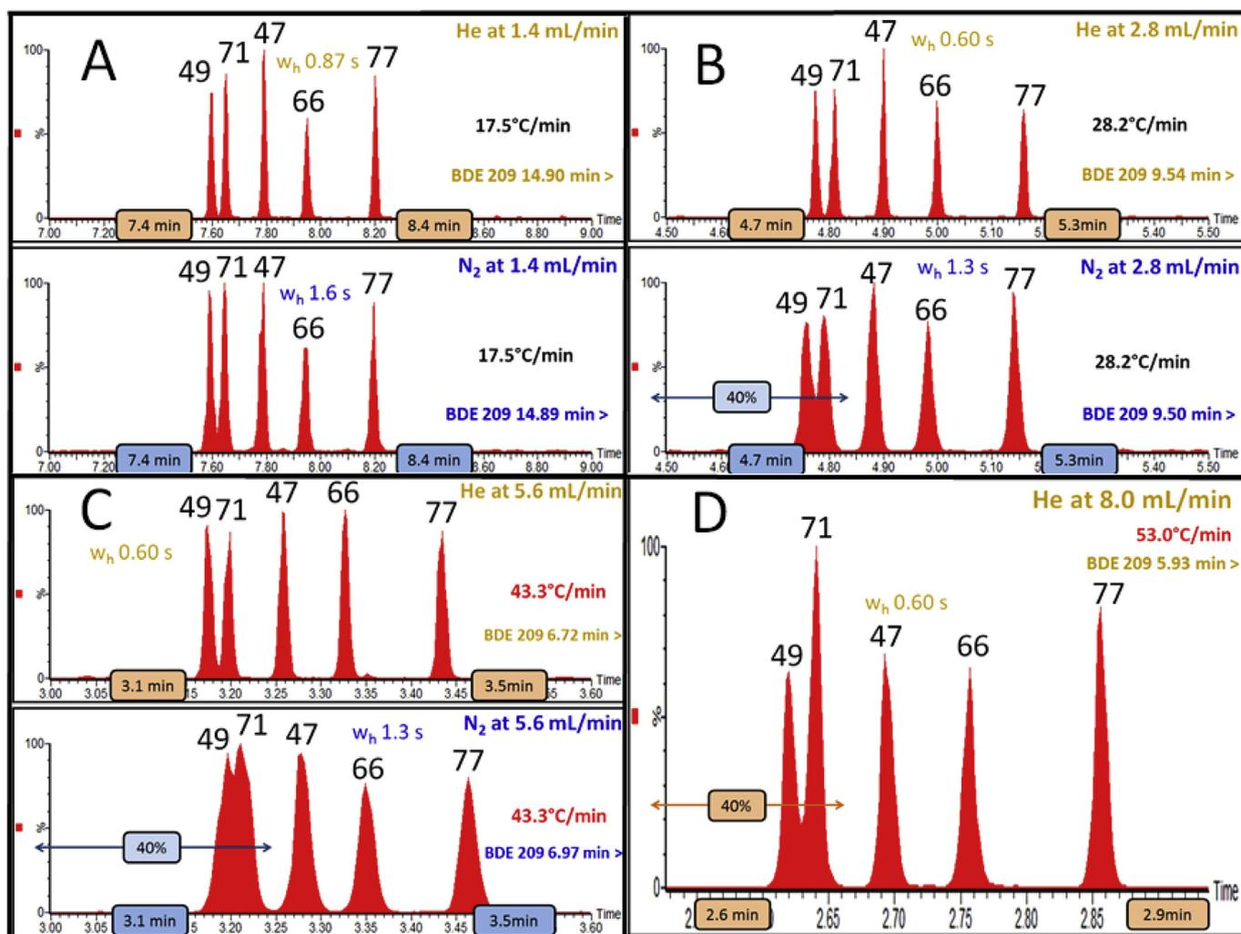
**Fig. 4.** Extracted ion chromatograms of tetra-BDEs using: (a) 1.4 mL/min of He (top) and N<sub>2</sub> (bottom); (b) 2.8 mL/min of He (top) and N<sub>2</sub> (bottom); (c) 5.6 mL/min of He (top) and N<sub>2</sub> (bottom); (d) 8.0 mL/min of He.
