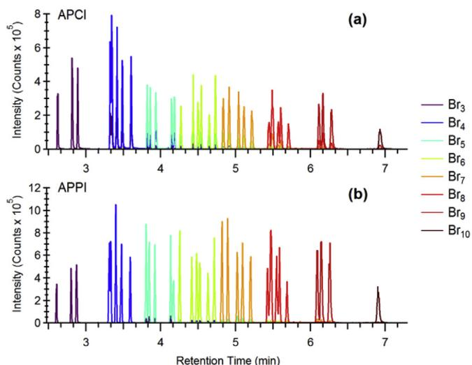
**Fig. 5.** Extracted ion chromatograms of (Br<sub>3</sub>-Br<sub>10</sub>)-BDEs obtained by: (a) GC-APCI; and (b) GC-APPI.
