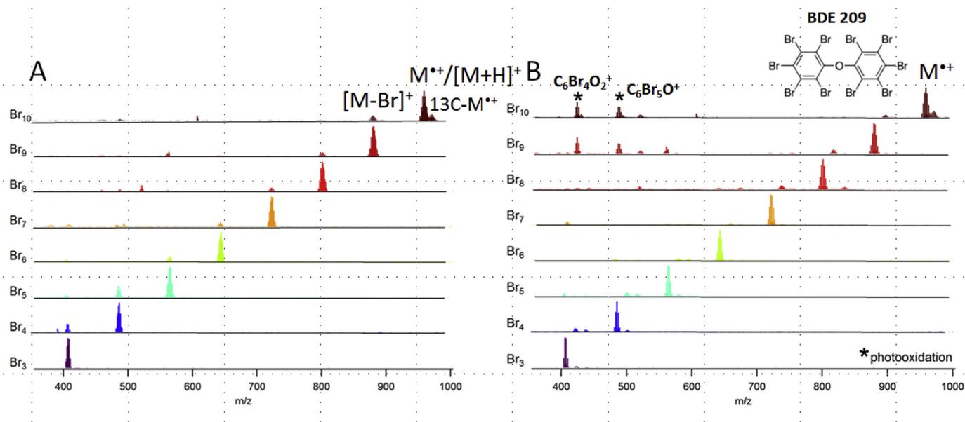
**Fig. 1.** (a) APCI and (b) APPI (Kr lamp) mass spectra of selected ( $\text{Br}_3$ - $\text{Br}_{10}$ ) PBDE congeners. The (\*) indicates the presence of photooxidation/dissociation products in the APPI spectra that are absent in the APCI spectra.
