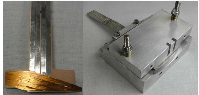
Fig. 6. (Left) Picture of terminal showing location of scarf and conductors on copper base. (Right) Terminal assembly soldering fixture with terminal prepared for fabrication.
