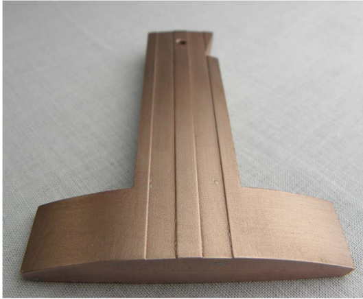
Fig. 4. Picture of the copper terminal base with channels machined for REBCO tape.
