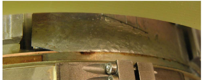
Fig. 7. Picture of terminal attachment soldering fixture with Nichrome heating strip over the joint area of the terminal.
