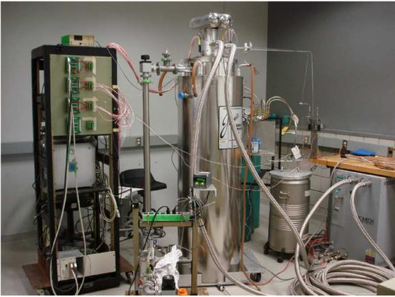
Fig. 7. Helium liquefaction system for the closed-loop cooling.
