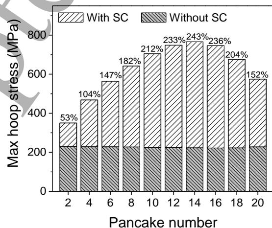
**Figure 12.** Maximum local hoop stresses in pancakes based on the discrete contact
