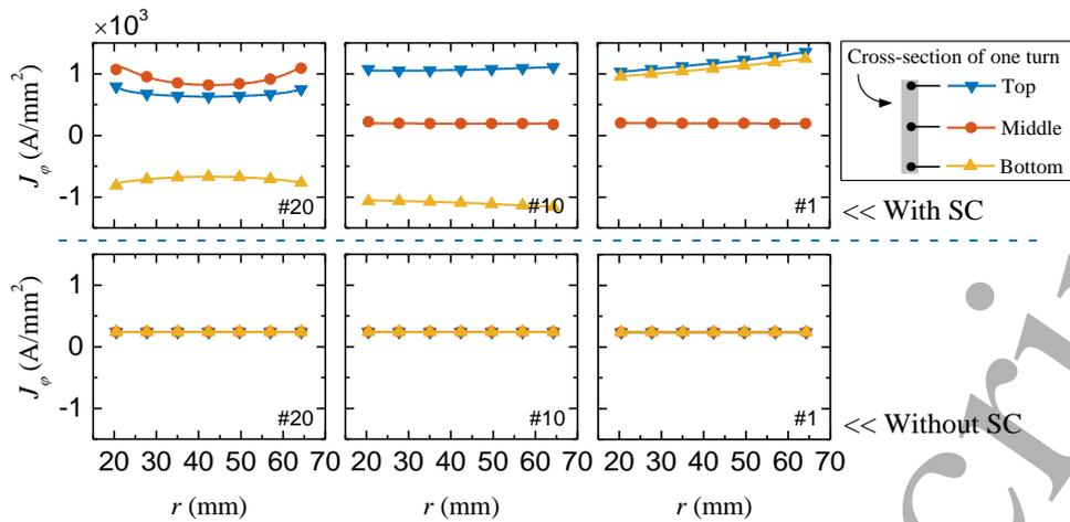
**Figure 8.** Profiles of the current density along the radial direction in pancakes #1, #10 and #20.
