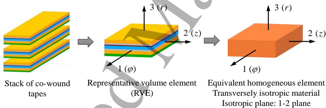
**Figure 3.** Equivalent homogeneous concept for the REBCO conductor/SS co-wound tape in a pancake.
