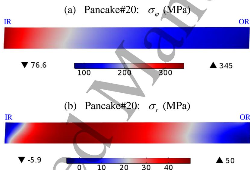
**Figure 13.** Distributions of (a) hoop stress and (b) radial stress in pancake #20 based on the bulk model, where the shielding current behavior is taken into account. A deformation scale factor of 40 is used here.
