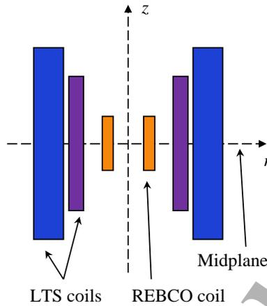
**Figure 1.** Schematic drawing of the superconducting coil system.
