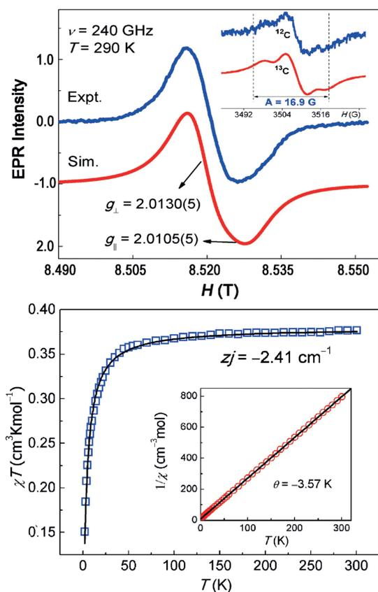
**Figure 1.** Top: EPR spectrum of compound **1**. Inset: EPR spectrum of <sup>13</sup>C-labeled **1** in the solid state (red: experimental, blue: simulation). Bottom: Temperature dependence of  $\chi_m T$  for compound **1** at 0.1 T. Inset:  $1/\chi_m$  vs.  $T$ . Solid lines represent the theoretical fits generated using the models discussed in the text.
