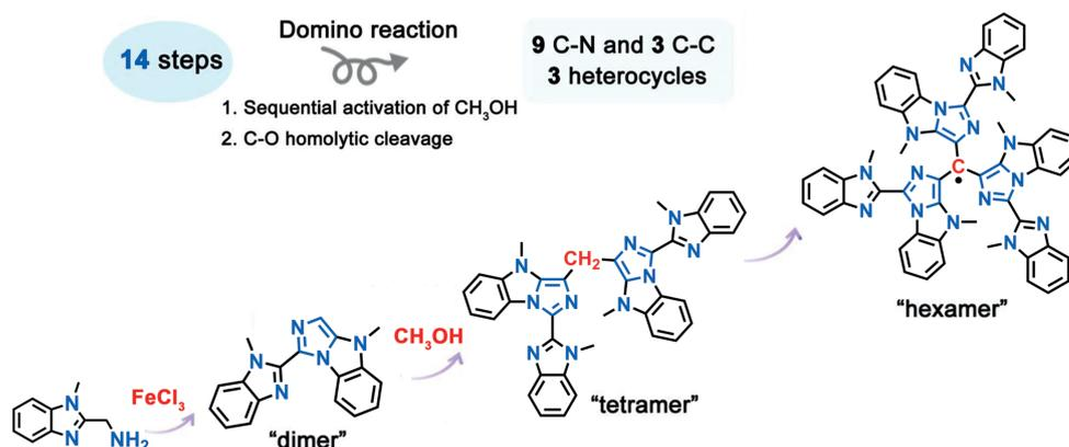
**Scheme 1.** The chemical structures of **L1**, “dimer” **3**, “tetramer” **2**, and “hexamer” **1** formed during the domino reaction leading to compound **1**.
