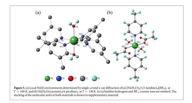
for the structural studies, but too small for thermodynamic measurements. The material is made up of distorted NiN<sub>4</sub>O<sub>2</sub> octahedra with four equatorial nitrogens donated by 3,5-lutidine, and two axial oxygens provided by water. The three bond angles between opposite donor atoms in the nickel octahedra are within the range  $176.95^{\circ}-179.17^{\circ}$ , and the *cis* N–Ni–O angle ranges between 87.7° and 92.3°.
