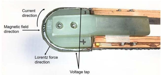
**Figure 3.** G-10 sample holder of 15 mm bend radius with soldered STAR wire # 4 mounted.
