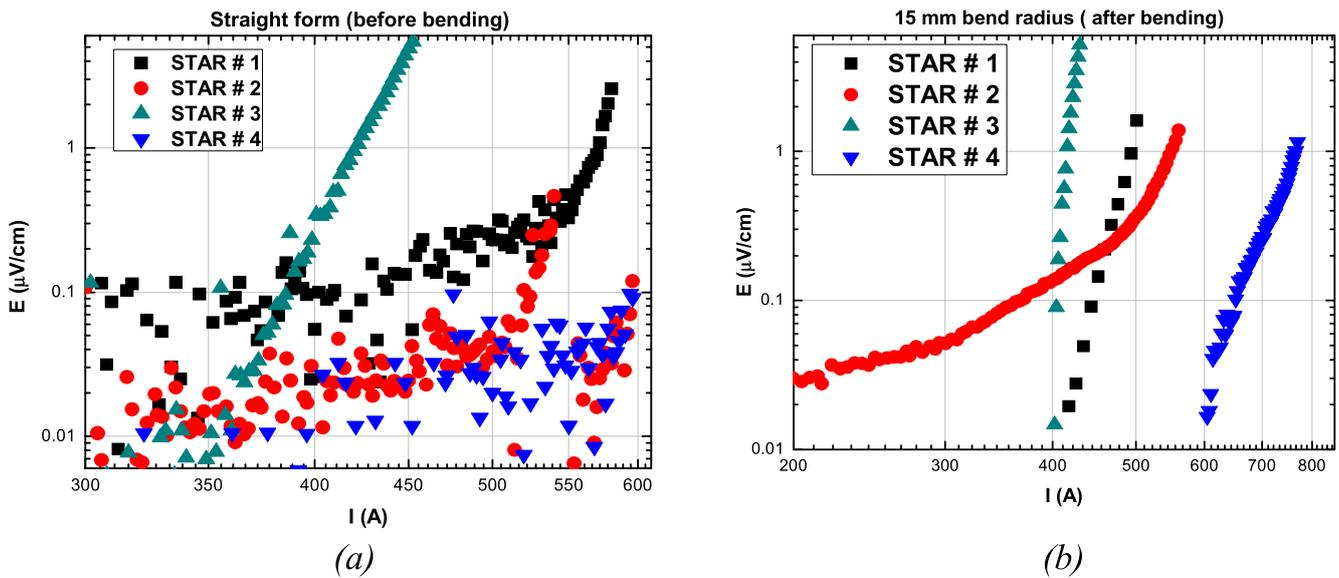
Figure 4.  $E$ - $I$  characteristics of the REBCO STAR wires at 77 K, self-field, in (a) straight form, and (b) 15 mm bending radius.
