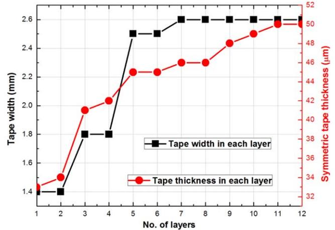
**Figure 2.** Width and thickness distribution of symmetric REBCO tapes used in REBCO STAR wire # 4.
