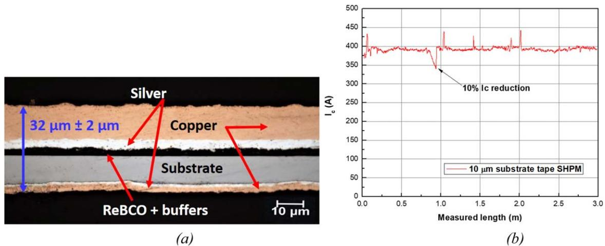
**Figure 1.** (a) Cross-section of symmetric REBCO tape with 10  $\mu\text{m}$  Hastelloy substrate, (b)  $I_c$  distribution over 3 m long, 12 mm wide, 10  $\mu\text{m}$  substrate REBCO tape before Cu plating.
