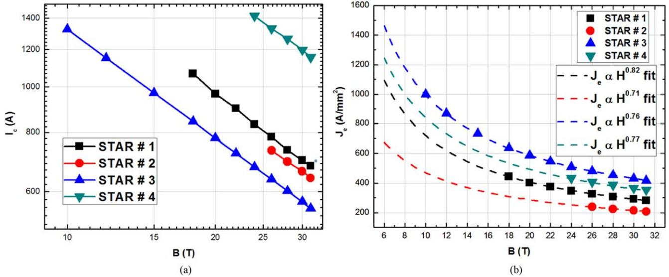
**Figure 5.** (a) Magnetic field dependence of  $I_c$  ( $0.5 \mu\text{V cm}^{-1}$  criterion was used for STAR wires #1 and #2,  $1 \mu\text{V cm}^{-1}$  criterion was used for STAR wires #3 and #4) and (b)  $J_e$  at different magnetic fields of STAR wires. (Dashed lines are a power-law fit to the data from 10 to 31.2 T.)
