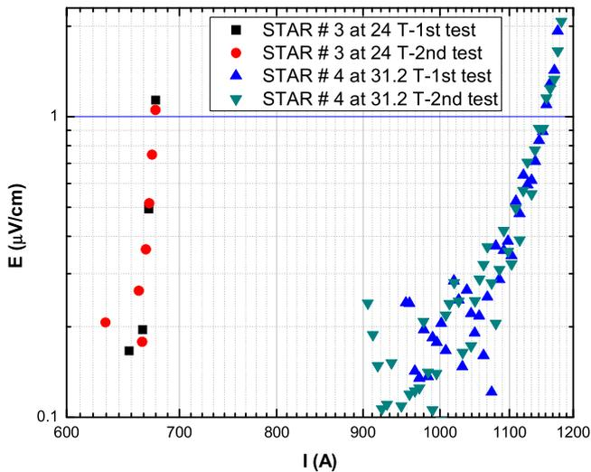
**Figure 6.**  $E$ - $I$  plot of STAR wire #3 at 24 T ( $F_L = 16.2 \text{ kN m}^{-1}$ ) and STAR wire #4 at 31.2 T ( $F_L = 36 \text{ kN m}^{-1}$ ) for two times measurement at same field.
