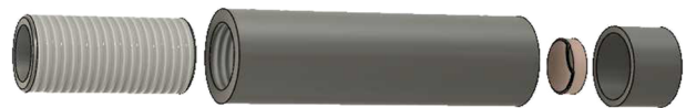
FIG. 5. The transducers for drive and detect are identical. They have four components: an SMA female barrel (left), an aluminum tube 8 mm \varnothing with 1/4-36 female threads at one end and a counterbore to fit the alumina cup at the other, a \varnothing 5 mm piezoelectric transducer 3 with any of several types of wrap-around electrodes, and an alumina cup that is 7.2 mm \varnothing , 6 mm bore, 5 mm long, 4 mm deep.
