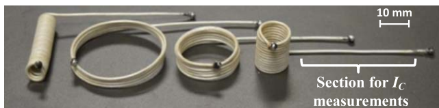
Figure 3. Picture of coils made from OP-PD wire after OP-HT. From left to right, 5, 30, 20, and 10 mm inside diameter coils. The total conductor length is 50 cm for each coil. Each coil has a 6 cm long straight section for I_C measurements. I_C measurements were also done on curved sections of the 30 mm diameter coil.
