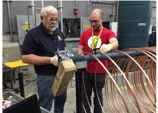
Fig. 9. ECT inspection of 13.7 mm diameter Glidcop AL60 precursor (about 100 m long). The encircling probe with frequency range of 100–500 MHz was used.
