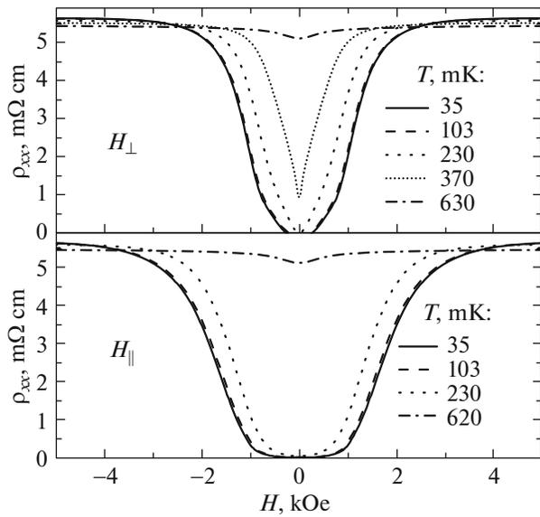
**Fig. 4.** Magnetic field dependences of the electrical resistance for two directions of the magnetic field, which was applied in the direction of  $0^\circ$  (magnetic field perpendicular to the plane of the sample, Fig. 4a) and  $90^\circ$  (magnetic field along the plane of the sample, perpendicular to the current, Fig. 4b) in the field up to 0.5 T. The numbers indicate the temperatures of the sample at which measurements were made.
