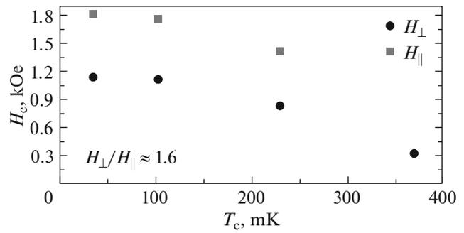
**Fig. 5.** The  $H_c$ – $T_c$  phase diagram constructed for  $\alpha = 1$  and  $\beta = 1$  according to Eq. (1), which corresponds to the Ginzburg–Landau theory.
