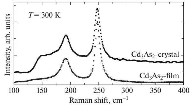
**Fig. 2.** The Raman shift of the curves for one of the  $\text{Cd}_3\text{As}_2$  samples at room temperature and the Raman shift of the curves for the  $\text{Cd}_3\text{As}_2$  single crystal at the same temperature, which has characteristic peaks at the points of 196 and  $245 \text{ cm}^{-1}$ .
