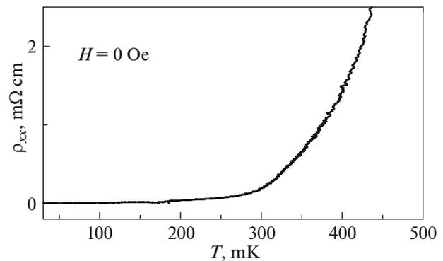
**Fig. 3.** Temperature dependences of the electrical resistance for the  $\text{Cd}_3\text{As}_2$  sample. The curve unambiguously indicates the observed transition to superconductivity.
