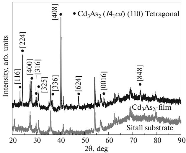
**Fig. 1.** Experimental X-ray diffraction patterns of the studied  $\text{Cd}_3\text{As}_2$  film on a sitall substrate. The peaks present confirm the existence of only the  $\alpha$ - $\text{Cd}_3\text{As}_2$  phase in the composition of the deposited film.
