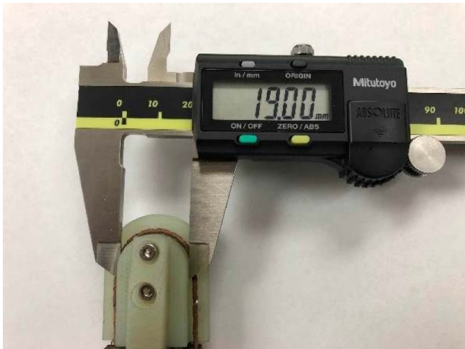
Figure 8. G-10 sample holder 19 mm in diameter with STAR wire # 10 mounted for 20 mm bend test.
