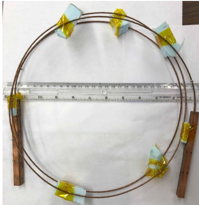
Figure 5. The 77 K self-field I_c test of STAR™ wire # 1 in the form of a 25 cm diameter coil.
