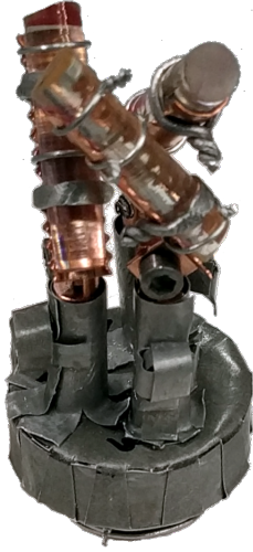
Figure A3. Three coaligned \text{Yb}_2\text{Ti}_2\text{O}_7 crystals used for the CNCS inelastic neutron scattering experiment. The base of the copper sample holder is wrapped in cadmium.
