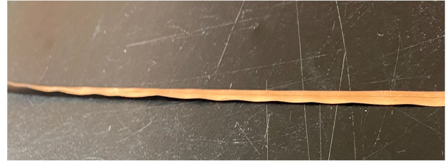
Fig. 3. The edges of the REBCO conductor are rippled after test in a test coil
