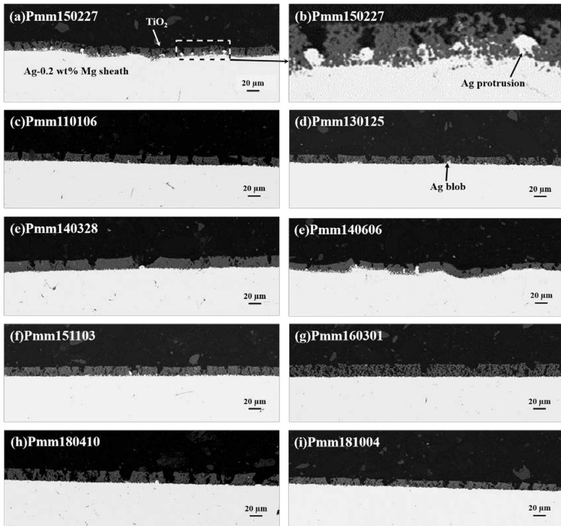
**Figure 2.** Longitudinal cross sections of different wires that underwent standard OPHT. A section of (a) is magnified in (b) for better demonstration of Ag protrusion. In (d), an arrow points to a Ag “blob”.
