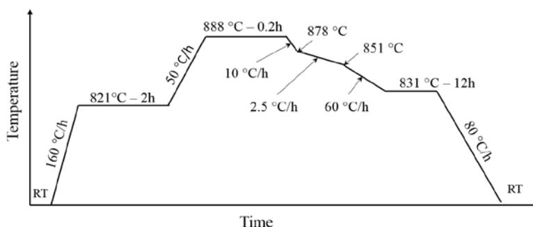
**Figure 1.** Standard heat treatment schedule for Bi-2212. For increased time in the melt samples, the cooling rate between 888 °C and 878 °C was reduced to 3.3 °C/h. The figure is not to the scale.
