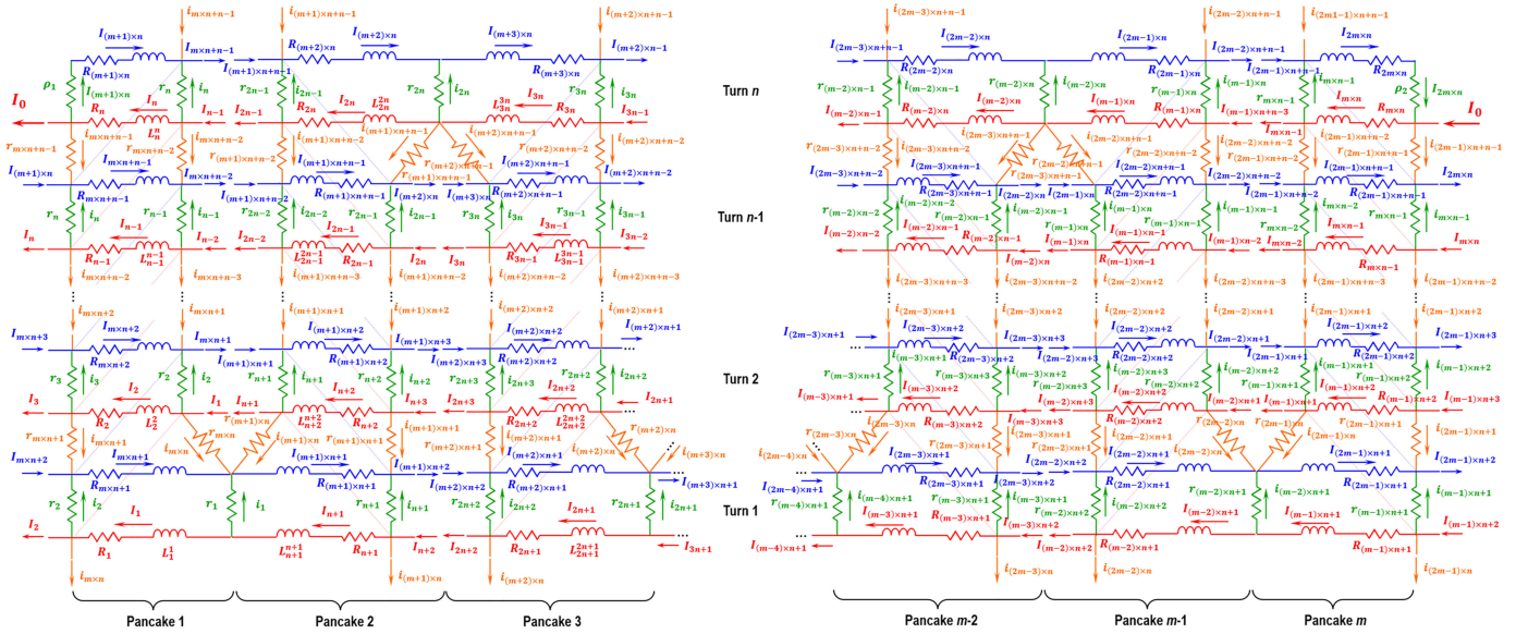
Fig. 3. A multi-rectangle planar grid as an equivalent electric circuit of a multi-module metal-insulation coil's subtle structure, i.e., with alternating REBCO-tape and normal-metal co-wind turns; 'm' pancakes totally with 'n' REBCO turns and 'n' co-wind turns per pancake.
