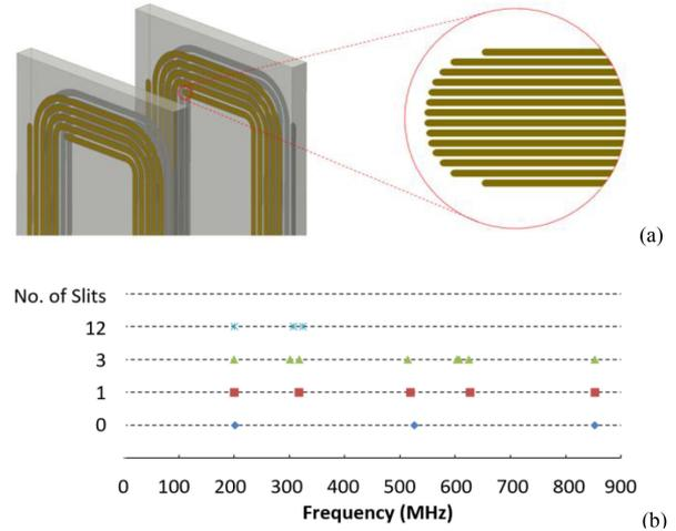
Fig. 2. Design of the  $^{13}\text{C}$  detection coils. (a) Pair of counter-wound spiral resonators. Each resonator employs two 4-turn YBCO spiral structures with opposite handedness coated onto either side of a sapphire substrate. To reduce magnetization, the HTS resonators are slit into 14 fine parallel fingerlets. The slits cause each mode to split into a family of modelets. (b) The modelets of one single-sided spiral coil as simulated using IE3D.
