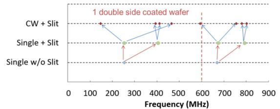
Fig. 3. Simulated modes of our current counter-wound (CW) spiral  $^{13}\text{C}$  detection coils. The modelets of the slit single spiral coil show further splitting when they are used in a CW spiral arrangement. Our simulation shows only a single mode near the  $^1\text{H}$  resonance of 600 MHz.
