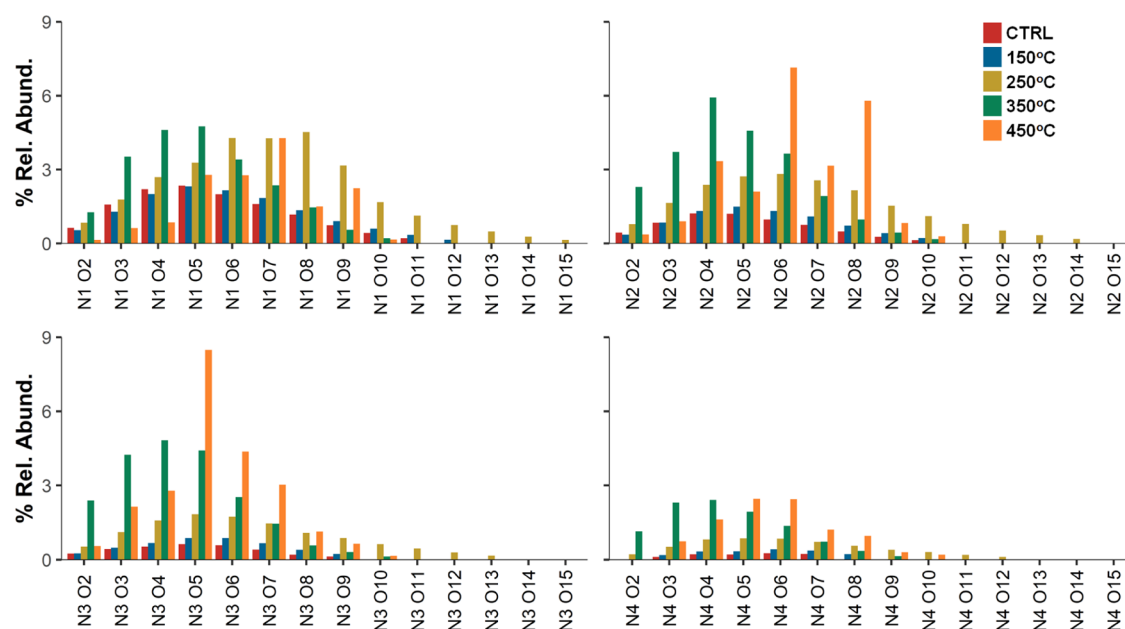
Figure 3. Percent relative abundance of CHNO classes in the unburnt (CTRL) and heated (150–450 °C) hydrophilic samples separated by the nitrogen and oxygen ( N_{1-4}O_{2-15} ) content. The N_{5}O_{2-15} and assignments from the hydrophobic fraction can be found in Figures S8 and S9, respectively.
